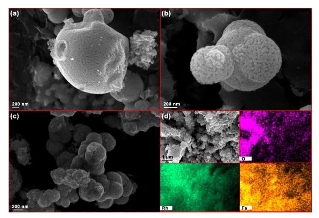
Fig. 4 (a and b) FESEM images of 3D spherical  $Rh_2O_3/Fe_2O_3$  structures obtained by decomposition of molecular precursor [Rh(acac)<sub>3</sub>Fe(hfac)<sub>2</sub>] (2) at 300 °C; (c) FESEM image of the Rh<sub>2</sub>O<sub>3</sub>/Fe<sub>2</sub>O<sub>3</sub> sample obtained at 400 °C showing partial agglomeration of spherical structures; (d) EDS elemental mapping of Rh<sub>2</sub>O<sub>3</sub>/Fe<sub>2</sub>O<sub>3</sub> material synthesized at 300 °C.
