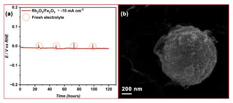
Fig. 6 (a) Chronopotentiometry response of  $Rh_2O_3/Fe_2O_3$  synthesized at 300 °C, recorded for 120 hours at the constant current density of  $\approx -10$  mA cm<sup>-2</sup> in 0.5 M  $H_2SO_4$ ; (b) FESEM image of the catalyst after the stability test.
