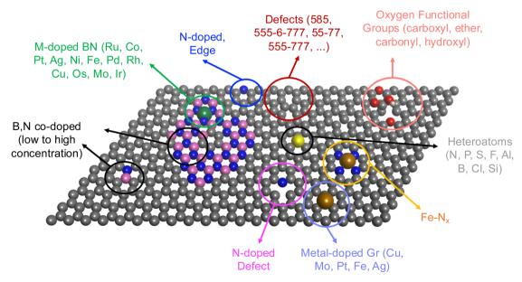
Fig. 1 Schematics of the active sites examined in this study as well as those reported in the literature for their high activity and selectivity toward 2e-ORR. The corresponding calculated and compiled adsorption energy values for ORR intermediates and relevant references are included in Tables S1-S4.
