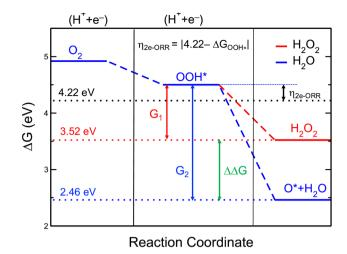
Fig. 2 Free energy diagram for 2e-ORR, illustrating the catalytic activity ( $\eta_{2e-ORR}$ ) and selectivity ( $\Delta\Delta G$ ) descriptors. Vertical black solid lines represent the steps of coupled proton-electron transfer. Black, red, and blue dotted lines represent the adsorption energy of the OOH\* intermediate for an ideal 2e-ORR catalyst, the free energy of  $H_2O_2$  in agueous solution, and the adsorption energy of O\* for an ideal 4e-ORR catalyst, respectively.
