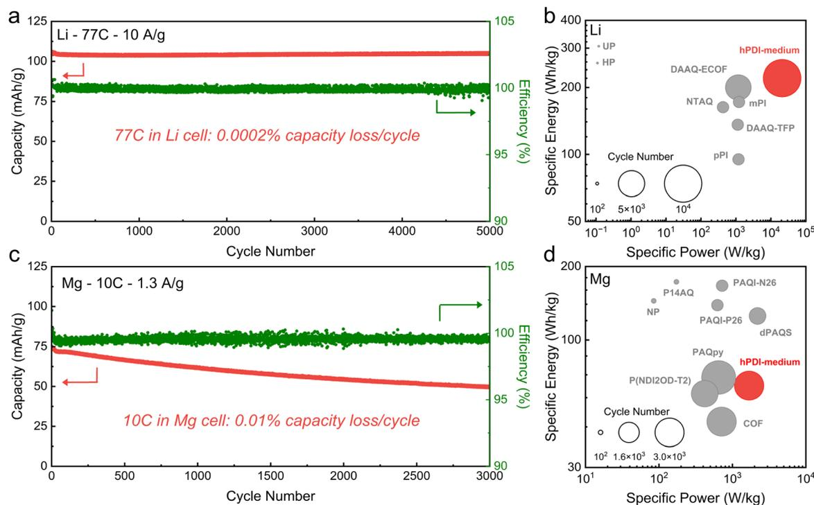
Fig. 5 Galvanostatic cycling performance of **hPDI-medium** in (a) Li batteries at 77 C for 5000 cycles and (c) Mg batteries at 10 C for 3000 cycles. Ragone plot comparing **hPDI-medium** with reported organic polymeric electrodes for (b) Li batteries and (d) Mg batteries. The circle size is the performance at maximum reported cycle number.
