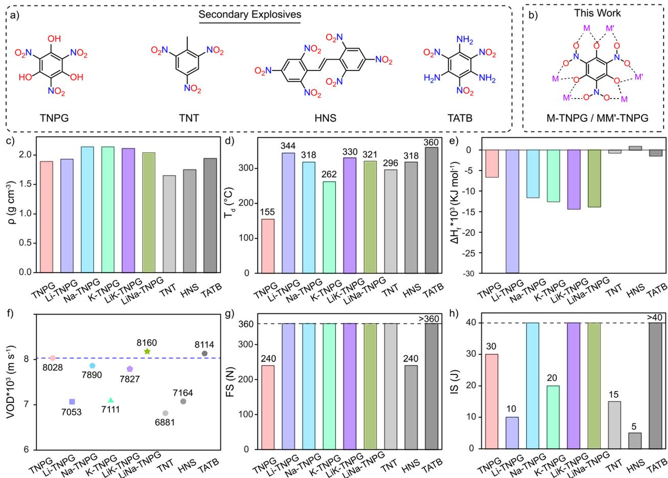
Fig. 5 (a) Literature reported secondary explosives.<sup>34</sup> (b) Strategy adopted in designing the secondary explosives in this work. The physico-chemical properties of the TNPG-based mono- and hetero-metallic coordination networks compared with the literature reported explosives: (c) Experimental density, (d) onset decomposition temperature, (e) heat of formation, (f) velocity of detonation (VOD), (g) friction, and (h) impact sensitivity.
