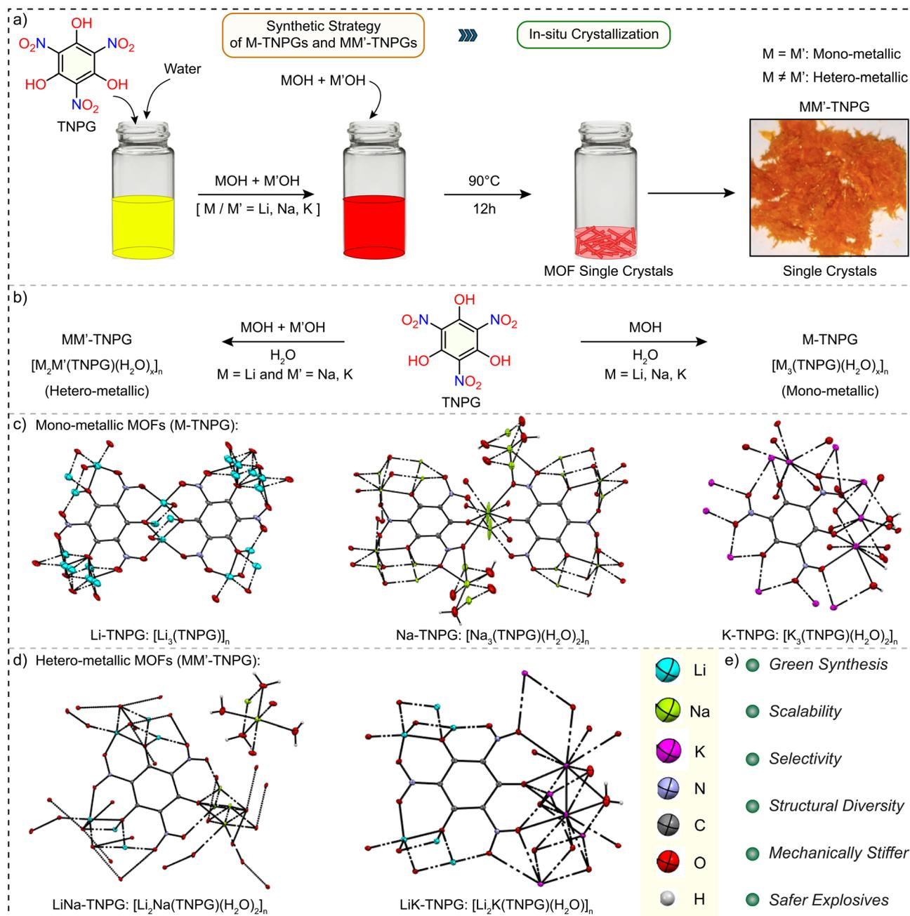
**Fig. 1** (a) Schematic representation of the synthetic methodologies and (b) general synthetic scheme of M-TNPGs and MM'-TNPGs (M/M' = Li, Na, and K). Single crystal X-ray diffraction structure of the (c) mono-metallic metal–organic networks (M-TNPGs: M = Li, Na, and K) and (d) hetero-metallic metal–organic networks (MM'-TNPG: MM' = LiNa and LiK). (e) Synthetic advantages and properties of the metal–organic networks.
