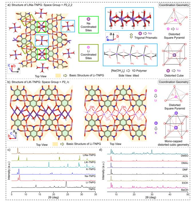
Fig. 3 Single crystal X-ray diffraction structures of MM'-TNPGs and the coordination geometries of M<sup>+</sup> ions: (a) LiNa-TNPG and (b) LiK-TNPG. (c) and (d) Powder X-ray diffraction patterns of as-synthesized M-TNPGs (M = Li, Na, and K) and MM' - TNPGs (MM' = LiK and LiNa) following thermoevaporative in situ crystallization and (d) LiNa-TNPG after treatment with solvents with a high dielectric constant ranging from ~24 to 47.
