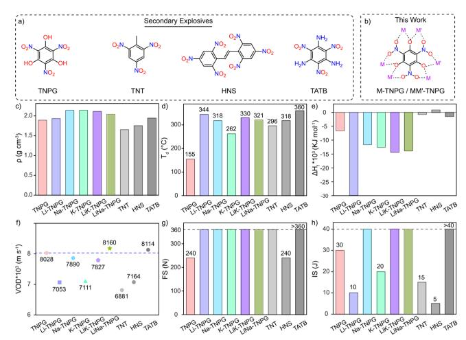
Fig. 5 (a) Literature reported secondary explosives.<sup>34</sup> (b) Strategy adopted in designing the secondary explosives in this work. The physicochemical properties of the TNPG-based mono- and hetero-metallic coordination networks compared with the literature reported explosives: (c) Experimental density, (d) onset decomposition temperature, (e) heat of formation, (f) velocity of detonation (VOD), (g) friction, and (h) impact sensitivity
