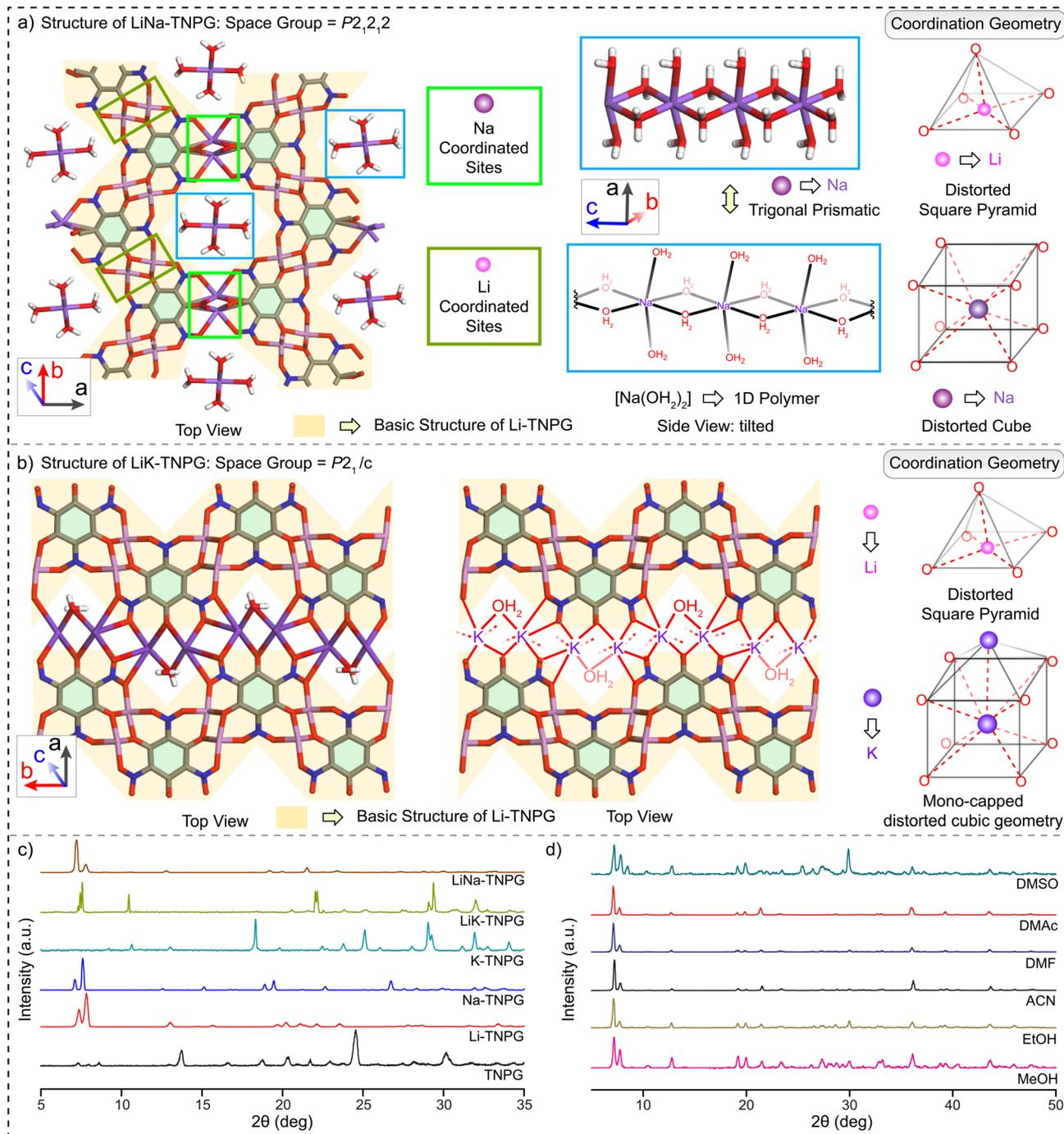
**Fig. 3** Single crystal X-ray diffraction structures of MM'-TNPBs and the coordination geometries of  $M^+$  ions: (a) LiNa-TNPG and (b) LiK-TNPG. (c) and (d) Powder X-ray diffraction patterns of as-synthesized M-TNPBs (M = Li, Na, and K) and MM'-TNPBs (MM' = LiK and LiNa) following thermo- evaporative *in situ* crystallization and (d) LiNa-TNPG after treatment with solvents with a high dielectric constant ranging from  $\sim 24$  to 47.
