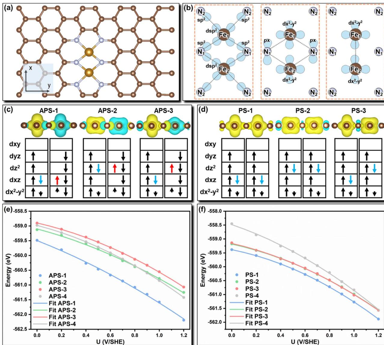
Fig. 2 (a) Model of Fe<sub>2</sub>N<sub>6</sub>. (b) Schematic diagram of Fe d orbital bonding in Fe<sub>2</sub>N<sub>6</sub>. (Dashed lines refer to the bonding interaction.) Spin density and d orbital occupation of several stable (c) APS states and (d) PS states of Fe<sub>2</sub>N<sub>6</sub>. (Smaller arrows refer to partial occupation.) Potential-dependent energies of several (e) APS states and (f) PS states of Fe<sub>2</sub>N<sub>6</sub>.
