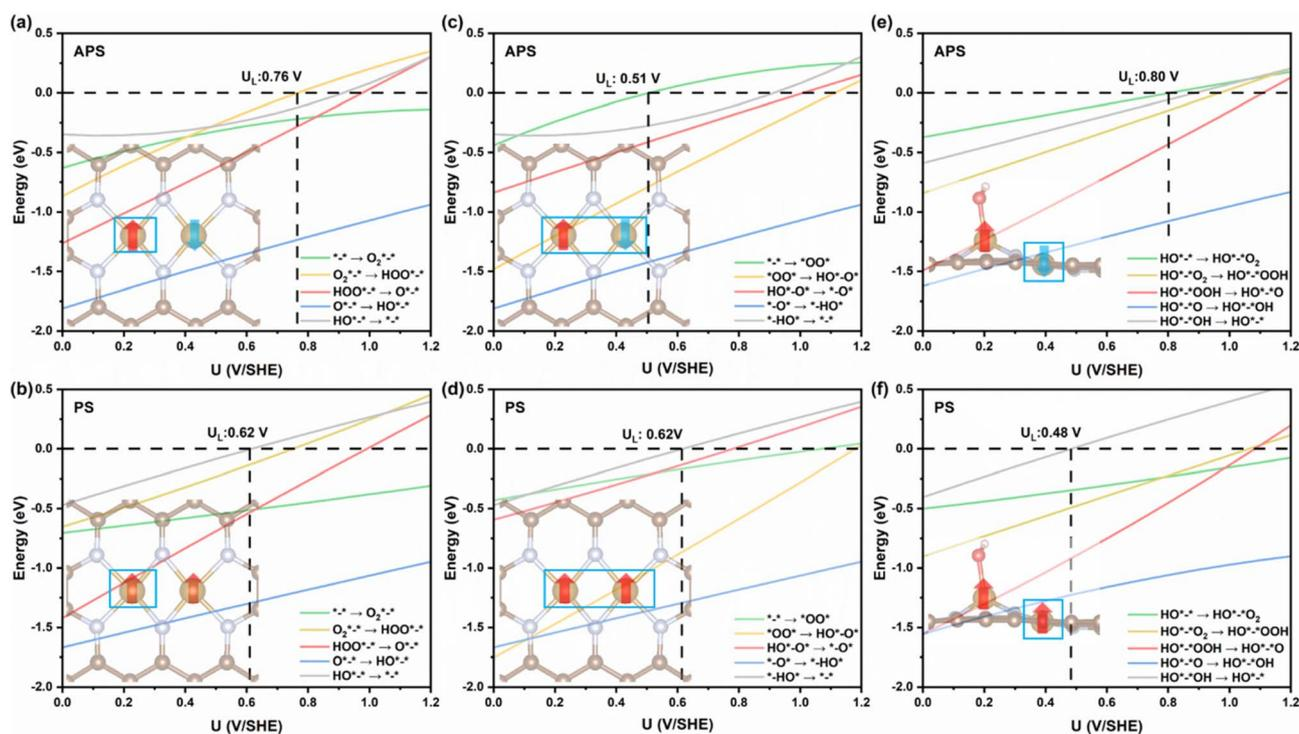
Fig. 4 Potential-dependent reaction free energy of the ORR at a single Fe site in (a) APS- and (b) PS- $\text{Fe}_2\text{N}_6$ . Potential-dependent reaction free energy of ORR at two Fe sites in (c) APS- and (d) PS- $\text{Fe}_2\text{N}_6$ . (The reaction path is shown in Fig. S13b.) Potential-dependent reaction free energy of ORR in (e) APS- and (f) PS- $\text{HO}^{*}\text{Fe}_2\text{N}_6$ . (The Fe atoms in the blue frame are the active sites.)
