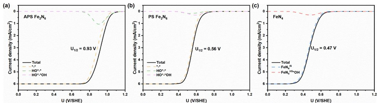
Fig. 5 Simulated ORR polarization current density in (a) APS- $\text{Fe}_2\text{N}_6$ , (b) PS- $\text{Fe}_2\text{N}_6$  and (c)  $\text{FeN}_4$ . The onset potential is 1.04 V, 0.67 V, and 0.61 V, respectively.
