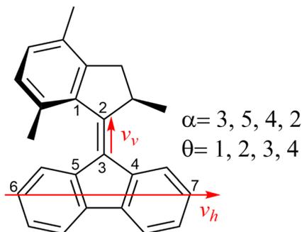
Fig. 3 Dihedral angles used to compute the PES and frame of reference employed. The vertical vector  $v_v$  is defined as the unit vector connecting the atoms 2 and 3. The horizontal vector  $v_h$  defines the directionality of the fluorene moiety and is defined as the unit vectors connecting the atoms 6 and 7.
