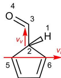
Fig. 5 Dihedral angle used to compute the PES and frame of reference employed. The torsional angle scanned to obtain the PES is defined by atoms 1–4. The vertical vector  $v_v$  is defined as the unit vector connecting the atoms 2 and 3. The horizontal vector  $v_h$  is defined as the unit vectors connecting the atoms 5 and 6, it describes the position of the cyclopentadiene with respect to the aldehyde.
