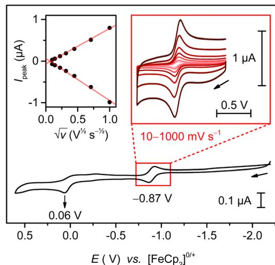
Fig. 5 Cyclic voltammogram of **3** in 0.1 M  $[\text{t}^{\text{Bu}}_4\text{N}][\text{PF}_6]$  in THF ( $10 \text{ mV s}^{-1}$ ), referenced to  $[\text{FeCp}_2]^{0/+}$  at 0.00 V. Insets show the reversible feature at  $-0.87$  V at scan-rates from  $10\text{--}1000 \text{ mV s}^{-1}$  (right) and a plot of the anodic/cathodic peak currents vs. the square root of the scan rate (top left inset).
