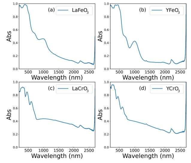
Fig. 6 UV-vis-NIR absorption spectra of synthesized samples measured in the range of 200–2700 nm: (a) LaFeO<sub>3</sub>, (b) YFeO<sub>3</sub>, (c) LaCrO<sub>3</sub>, and (d) YCrO<sub>3</sub>.
