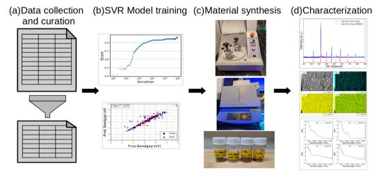
Fig. 1 Proposed workflow for materials design. (a) Data collection and curation. (b) Machine learning and descriptor search. (c) Materials synthesis in the experiment. (d) Materials characterization.
