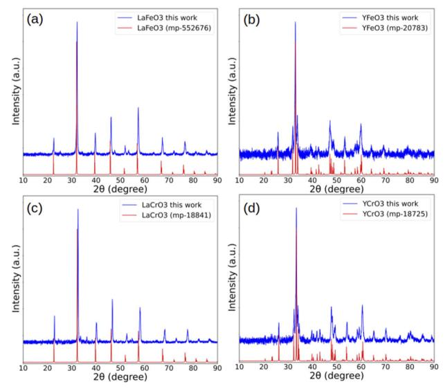
Fig. 4 Comparison of experimental and simulated X-ray diffraction (XRD) patterns for the synthesized perovskite oxides: (a)  $LaFeO_3$ , (b)  $YFeO_3$ , (c)  $LaCrO_3$ , and (d)  $YCrO_3$ . Experimental patterns (blue) are shown along with simulated patterns (red) based on CIF files for the target compounds obtained from the Materials Project database.
