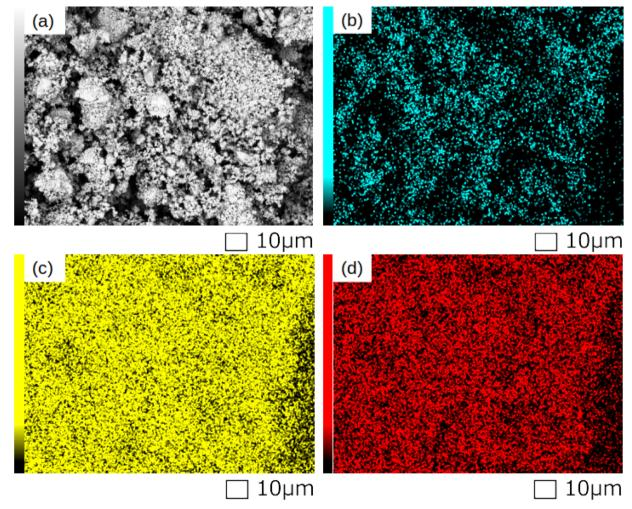
Fig. 5 SEM image and elemental maps of LaFeO<sub>3</sub> obtained by SEM-EDS. (a) SEM image, (b) O (K-line), (c) La (L-line), and (d) Fe (K-line).
