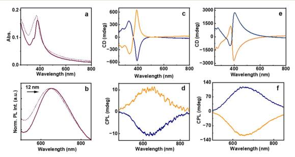
Fig. 3 (a) UV-vis and (b) PL spectra of the Au clusters synthesized at pH 4.2 (dotted trace) and 5.9 (solid trace). (c and e) CD and (d and f) CPL spectra of the Au clusters synthesized in the (c and d) absence of base (pH = 4.2) and (e and f) the inverted spectra upon in situ base addition (pH = 5.9). Blue and orange traces correspond to the clusters synthesized using L- and D-cysteine, respectively.
