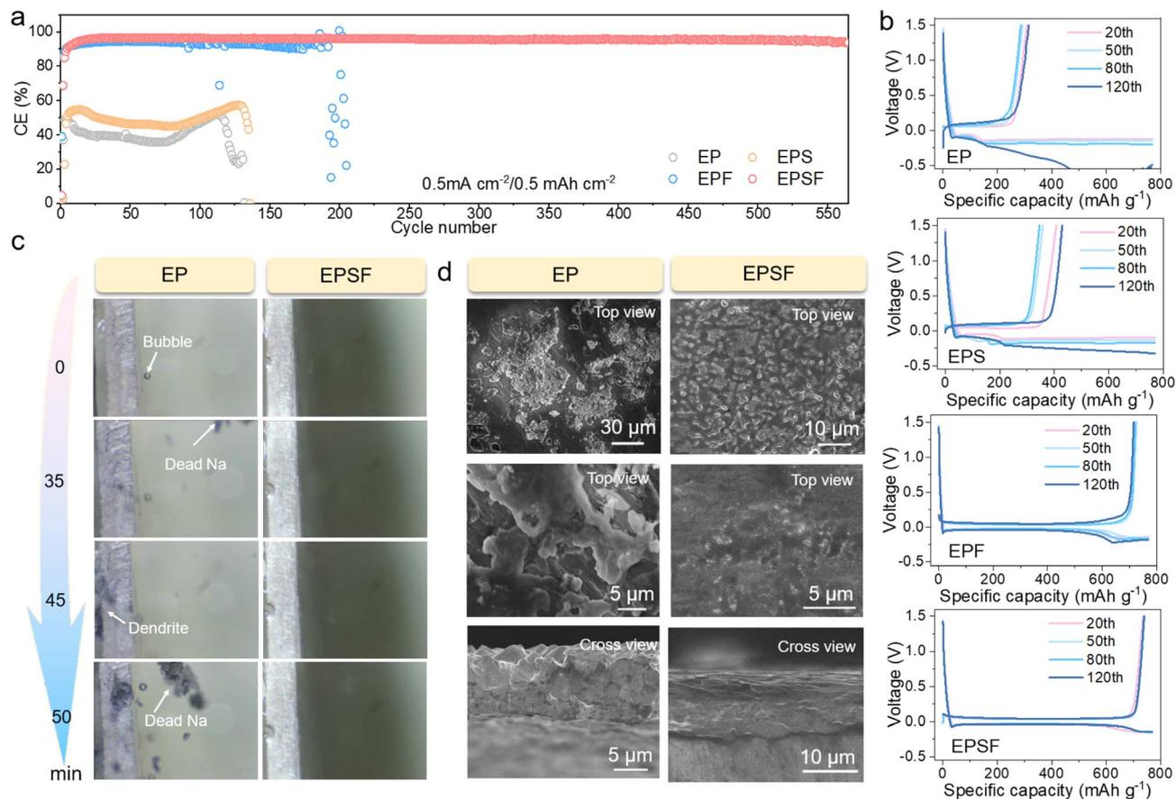
Fig. 3 Electrochemical performance of Na||Cu cells and interface evolution of the Na metal anode. (a) CE and (b) GCD curves of Na||Cu cells with different electrolytes. (c) *In situ* optical microscopy of the electrode–electrolyte interface on the Na anode with EP and EPSF electrolytes. (d) SEM images of Cu anodes of Na||Cu cells after the 50th cycle.
