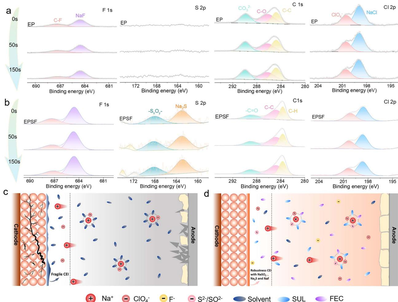
Fig. 6 Interface characteristics of the cathode with electrolytes and the schematic of the bidirectional interfacial engineering strategy. F 1s, S 2s, C 1s, and Cl 2p XPS spectra of the NVP cathodes with (a) EP and (b) EPSF electrolytes after 180 cycles. Schematic of the cathode stabilizing mechanism in (c) EP and (d) EPSF electrolytes.
