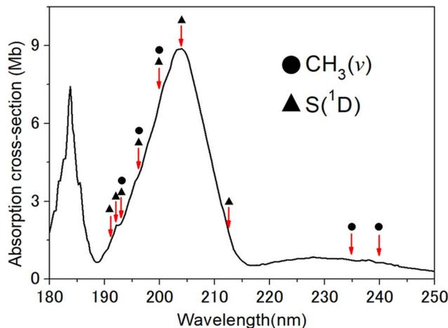
Fig. 1 Room temperature absorption spectrum of CH<sub>3</sub>SH (after ref. 27 and 29), with the photolysis wavelengths investigated in the present work marked and labelled to show the species probed at each wavelength.
