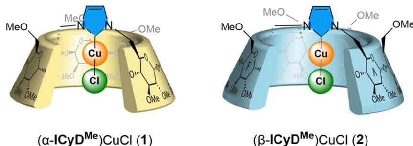
**Fig. 1** Water-soluble CD–NHC–copper(i) complexes [(α-ICyD<sup>Me</sup>)CuCl] (**1**) and [(β-ICyD<sup>Me</sup>)CuCl] (**2**) based on permethylated cyclodextrins, used in this study.
