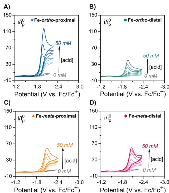
Fig. 3 Catalytic cyclic voltammograms for (A) **Fe-ortho-proximal**, (B) **Fe-ortho-distal**, (C) **Fe-meta-proximal**, and (D) **Fe-meta-distal** with increasing amounts of 3,5-bis(trifluoromethyl) phenol. Conditions: 0.25 mM catalyst, 0, 5, 10, 20, 30, and 50 mM 3,5-bis(trifluoromethyl) phenol, 1 atm  $\text{CO}_2$  (0.28 M), and 0.1 M TBAPF<sub>6</sub> in MeCN.
