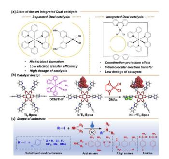
Fig. 1 (a) State-of-the-art integrated dual catalysis (left, separated dual catalysis; right, integrated dual catalysis). (b) Illustration of the  $\rm Ti_6$ -cluster based dual catalyst design strategy; the red block is the [Ir(ppy)<sub>2</sub>] complex in Ir/Ti<sub>6</sub>-Bpca, and the green block is NiCl<sub>2</sub> in Ni-Ir/Ti<sub>6</sub>-Bpca. (c) Available substrates for the established light-driven C-N cross-coupling strategy.
