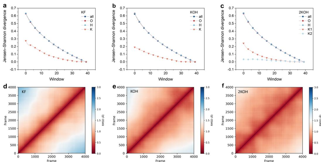
Fig. 2 Stability assessment of the three studied systems. (a)–(c) Jensen–Shannon divergence of all atoms, O, H, and K atoms over the last 2.0 ps (equivalent to 4000 frames) of the AIMD simulation trajectories for the KF, KOH, and 2KOH interface models at  $U = -0.65$  V vs. RHE. The window is set to 100. (d)–(f) Pairwise RMSD of all atoms in the KF, KOH, and 2KOH interface models.
