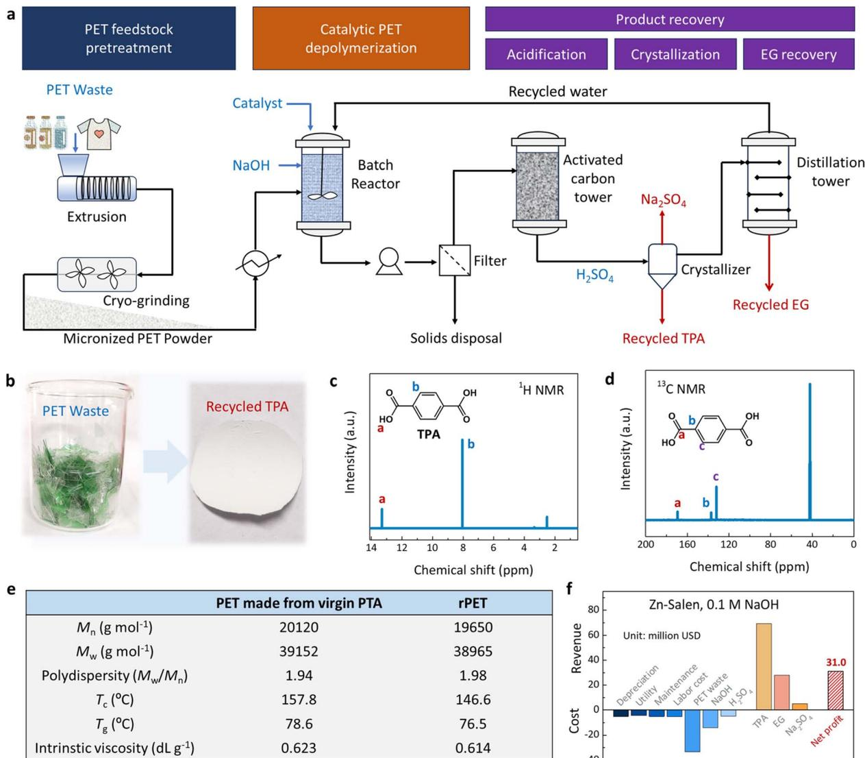
Fig. 7 PET recycling process, techno-economic analysis. (a) Simplified flow diagram of the PET recycling process over Zn-Salen/C. (b) TPA monomers obtained by recycling. (c) <sup>1</sup>H NMR spectrum and (d) <sup>13</sup>C NMR spectrum of recovered TPA. (e) Comparison of rPET made from the recycled PTA with the PET made from virgin PTA. (f) Techno-economic analysis of processing 100 thousand tons of waste PET annually based on this biomimetic catalytic system.
