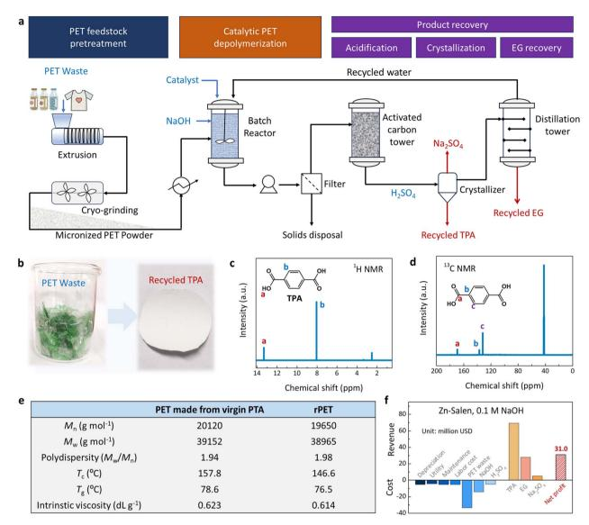
Fig. 7 PET recycling process, techno-economic analysis. (a) Simplified flow diagram of the PET recycling process over Zn-Salen/C. (b) TPA monomers obtained by recycling. (c) <sup>1</sup>H NMR spectrum and (d) <sup>13</sup>C NMR spectrum of recovered TPA. (e) Comparison of rPET made from the recycled PTA with the PET made from virgin PTA. (f) Techno-economic analysis of processing 100 thousand tons of waste PET annually based on this biomimetic catalytic system.
