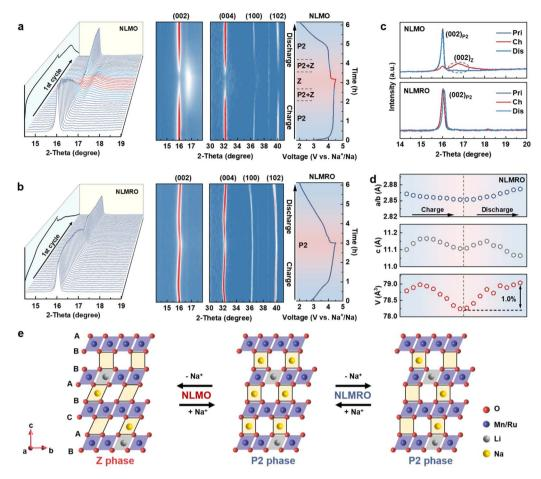
Fig. 4 Structure evolution of NLMO and NLMRO. *In situ* XRD patterns of (a) NLMO and (b) NLMRO during the first cycle at 0.2 C. (c) *In situ* XRD patterns of the (002) peak of NLMO and NLMRO in different states of charge. (d) Variation of unit cell parameters *a/b*, *c* and *V* for NLMRO. (e) Schematic illustration of the phase transition processes of NLMO and NLMRO.
