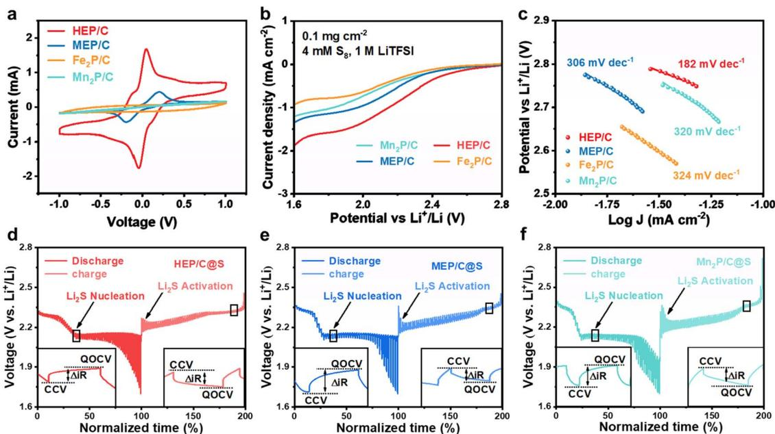
Fig. 3 (a) CV profiles of symmetric cells at a  $1 \text{ mV s}^{-1}$  scan rate. (b) LSV curves for sulfur reduction reaction activity comparison. (c) Tafel plots derived from LSV data. (d)–(f) GITT voltage profiles demonstrating (d) HEP/C, (e) MEP/C, and (f)  $\text{Mn}_2\text{P/C}$ .
