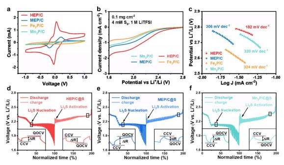
Fig. 3 (a) CV profiles of symmetric cells at a 1 mV s<sup>-1</sup> scan rate. (b) LSV curves for sulfur reduction reaction activity comparison. (c) Tafel plots derived from LSV data. (d)–(f) GITT voltage profiles demonstrating (d) HEP/C, (e) MEP/C, and (f) Mn<sub>2</sub>P/C.
