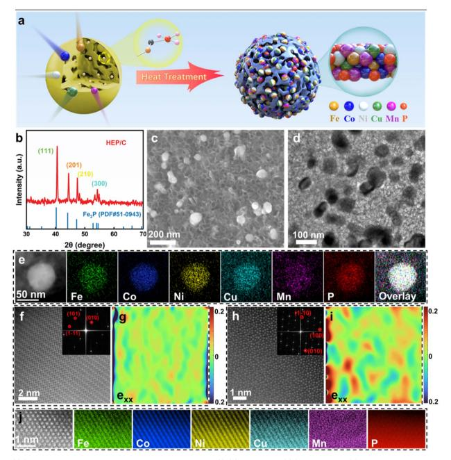
Fig. 1 (a) Schematic illustration of the synthesis mechanism for HEP/C. (b) XRD pattern, (c) SEM image, and (d) TEM image of the as-prepared HEP/C. (e) HAADF image and corresponding EDS element mapping of HEP/C. (f) and (h) STEM image viewed along the [-101] and [001] zone axis and (g) and (i) corresponding strain distribution maps. (j) Atomic-resolution elemental mapping of HEP/C.
