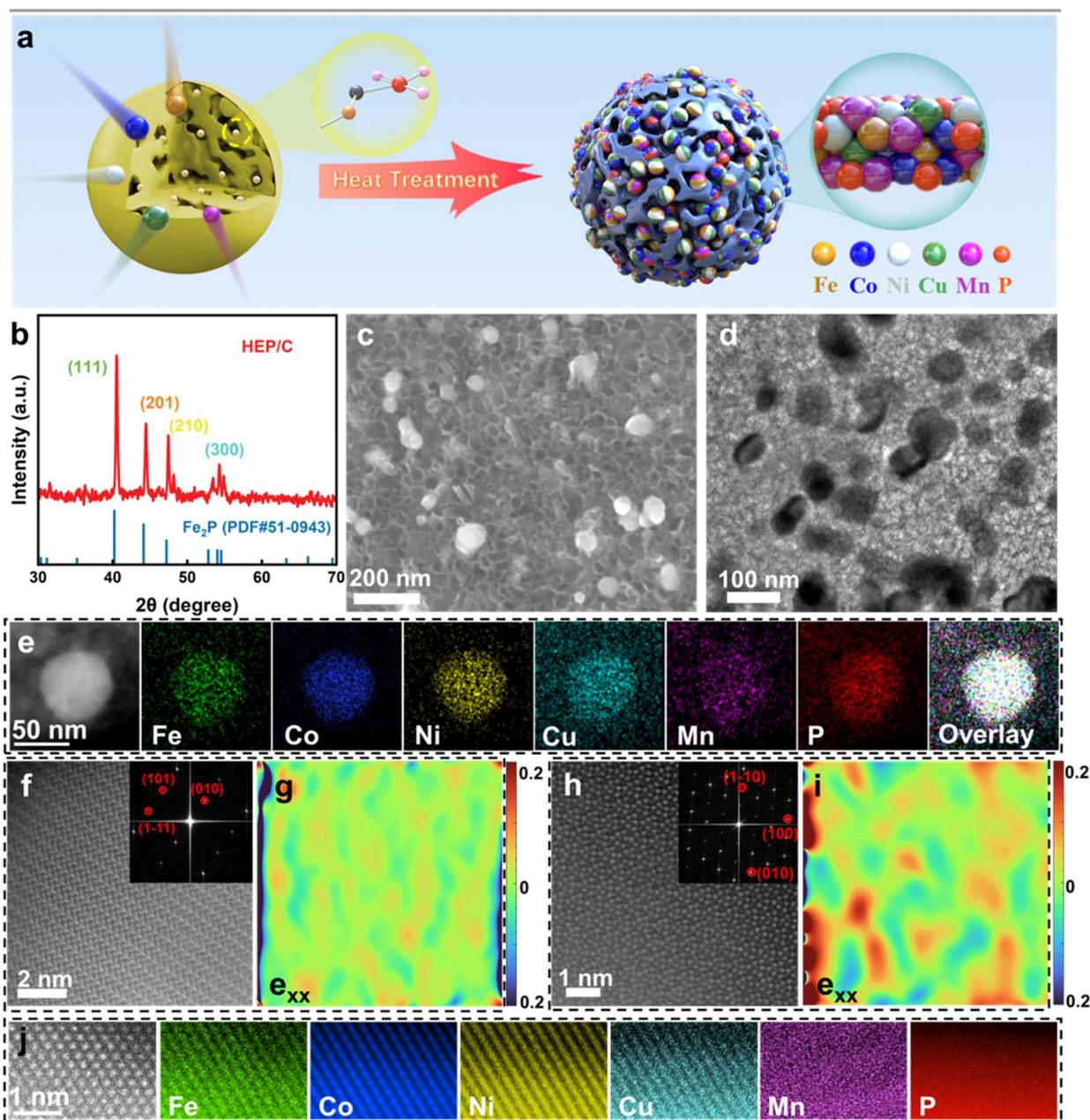
**Fig. 1** (a) Schematic illustration of the synthesis mechanism for HEP/C. (b) XRD pattern, (c) SEM image, and (d) TEM image of the as-prepared HEP/C. (e) HAADF image and corresponding EDS element mapping of HEP/C. (f) and (h) STEM image viewed along the  $[-101]$  and  $[001]$  zone axis and (g) and (i) corresponding strain distribution maps. (j) Atomic-resolution elemental mapping of HEP/C.
