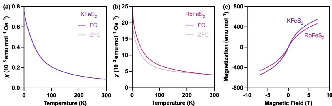
Fig. 4 Magnetic characterizations of  $\text{KFeS}_2$  and  $\text{RbFeS}_2$  nanowires. (a and b) Temperature-dependent zero-field-cooled (ZFC) and field-cooled (FC) magnetic susceptibility ( $\chi$ ). (c) Field-dependent magnetization at 5 K.
