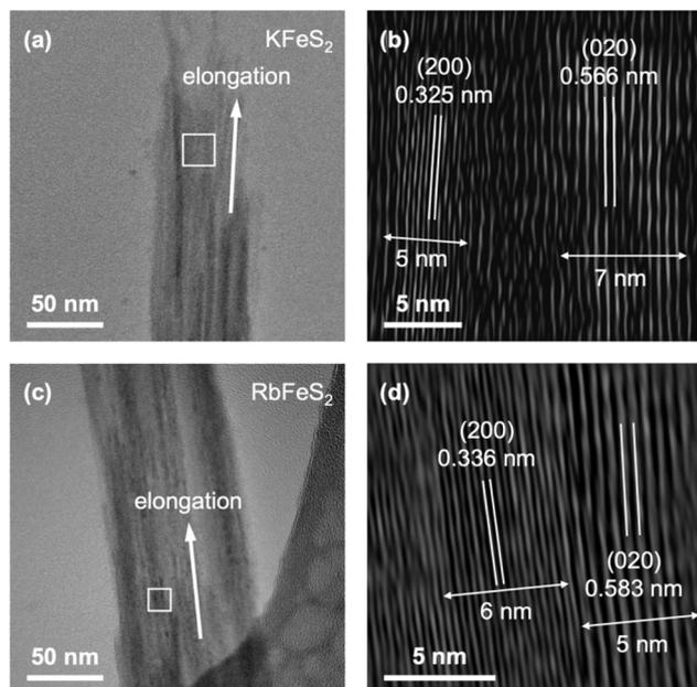
Fig. 2 (a and c) TEM images of a bundle of (a)  $\text{KFeS}_2$  and (c)  $\text{RbFeS}_2$  nanowires. (b and d) FFT-filtered magnified sections of the white boxed regions in (a) and (c), respectively, showing  $ac$  and  $bc$  plane spacings parallel to the nanowire elongation direction. Unfiltered images are shown in Fig. S3a and b.
