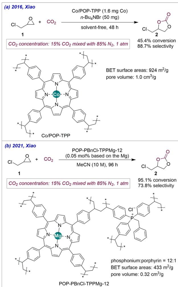
Scheme 2 Co and Mg/porphyrin ligand polymers catalyse the conversion of low-concentration CO<sub>2</sub>.
