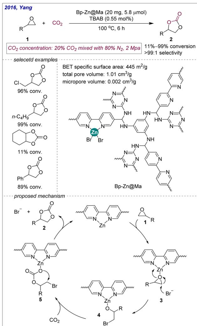
Scheme 3 Bp-Zn@MA catalyses the conversion of low-concentration CO<sub>2</sub>.
