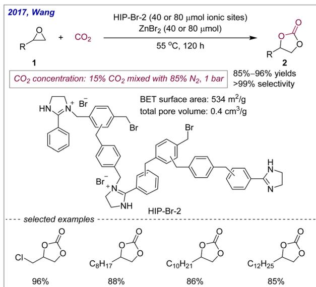
Scheme 5 HIP-Br-2 catalyses the conversion of low-concentration CO<sub>2</sub>.
