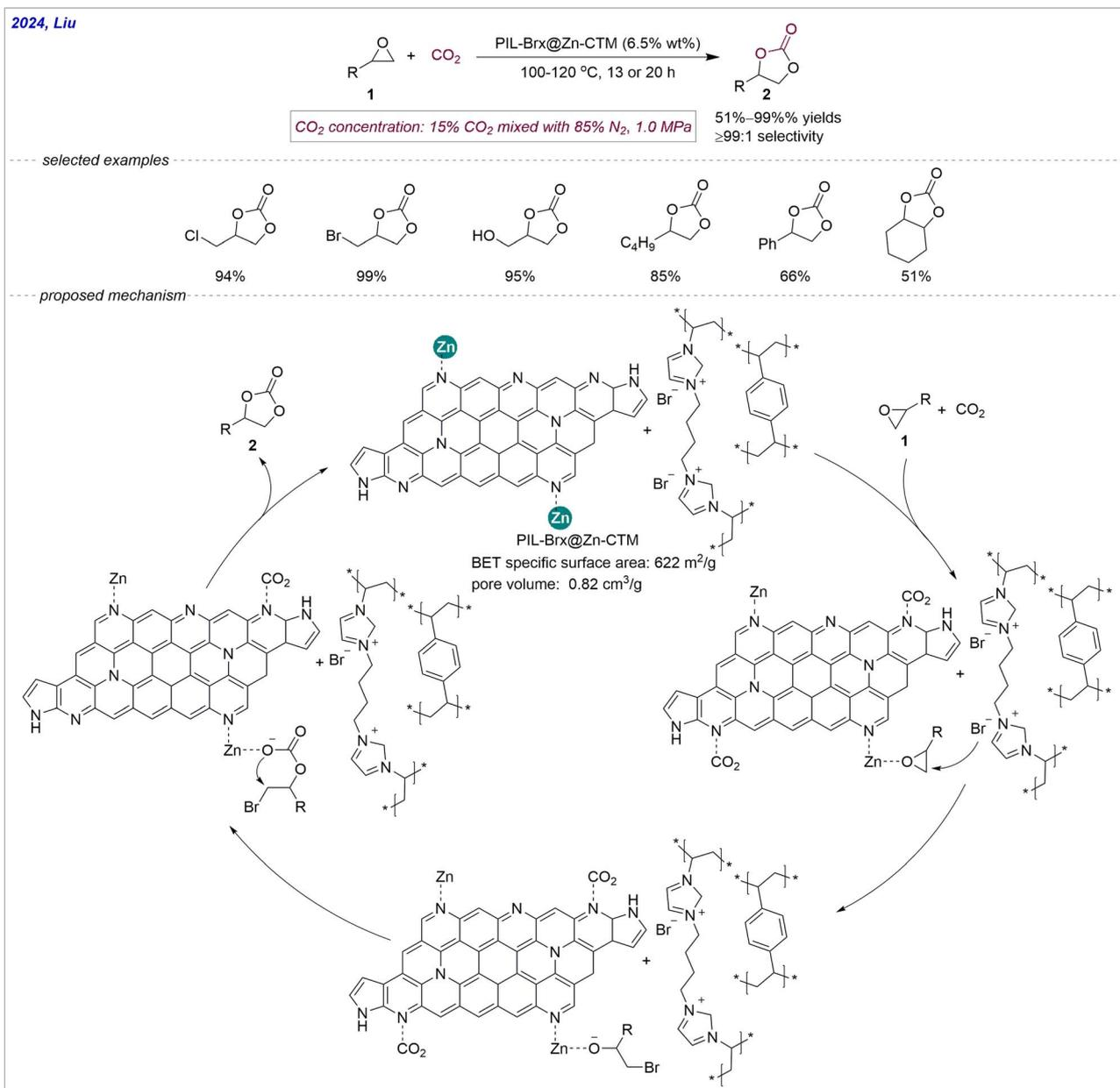
Scheme 4 Poly(ionic liquid)@porous carbon nanocomposites for the capture and *in situ* conversion of low-concentration CO<sub>2</sub>.
