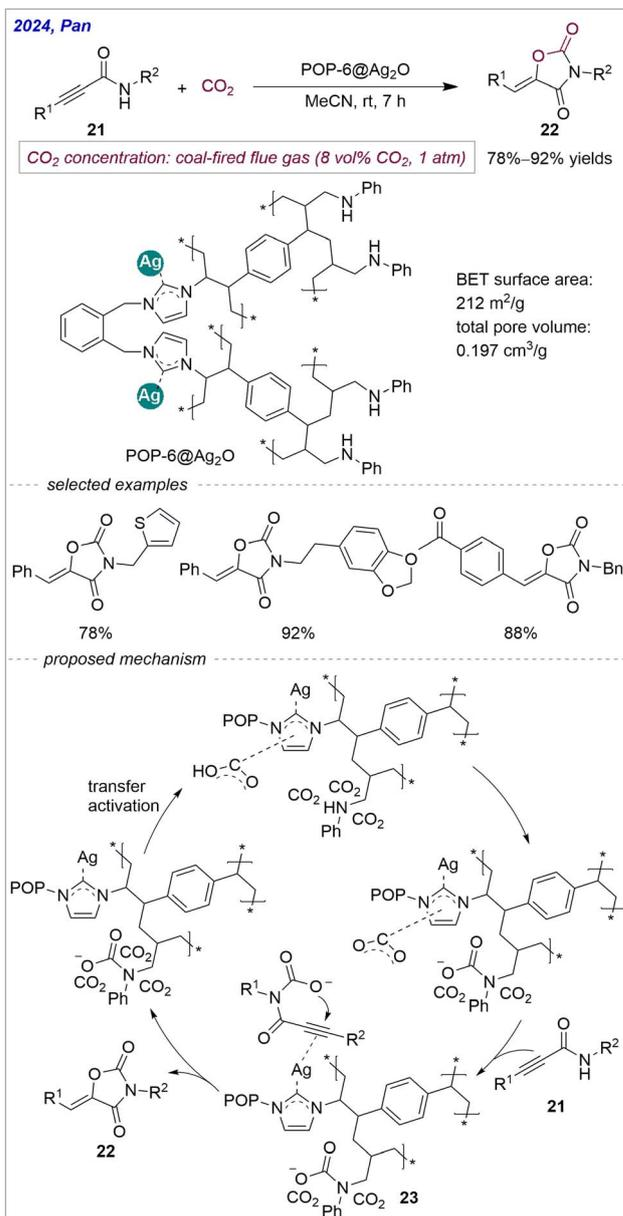
Scheme 10 POP-6@Ag<sub>2</sub>O catalyses CO<sub>2</sub> conversion in coal-fired flue gas.
