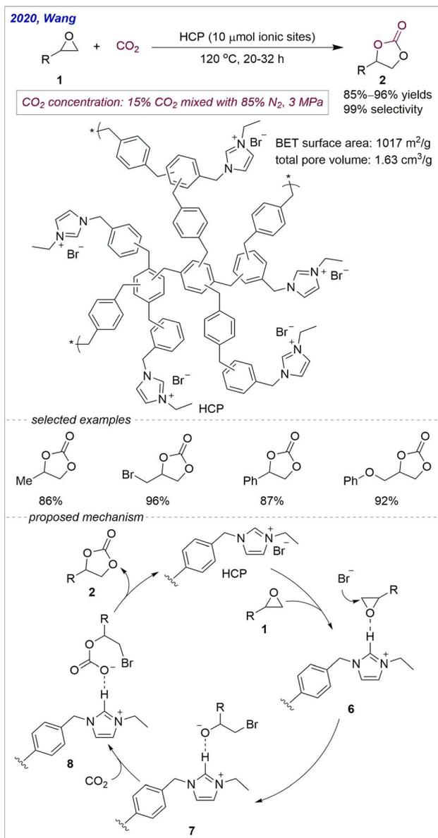
Scheme 6 HCP catalyses the conversion of low-concentration CO<sub>2</sub>.
