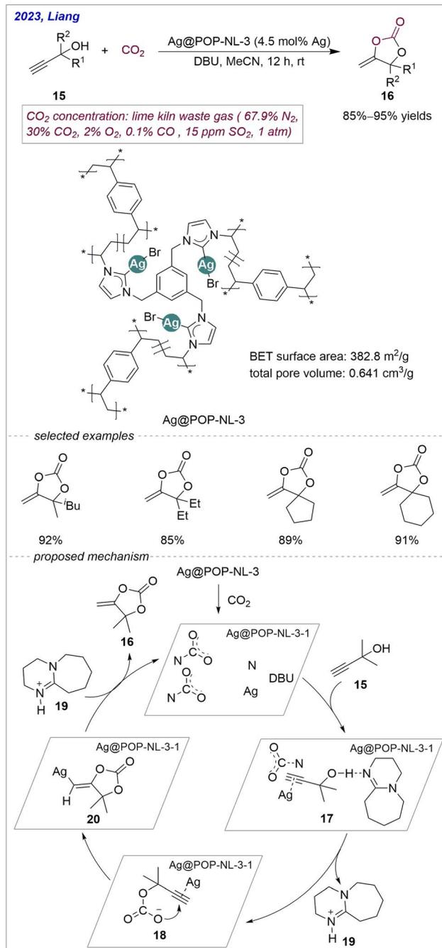
Scheme 9 Ag@POP-NL-3 catalyses CO<sub>2</sub> conversion in lime kiln waste gas.
