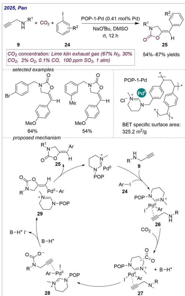
Scheme 11 POP-1-Pd catalyses  $\text{CO}_2$  conversion in lime kiln exhaust gas.
