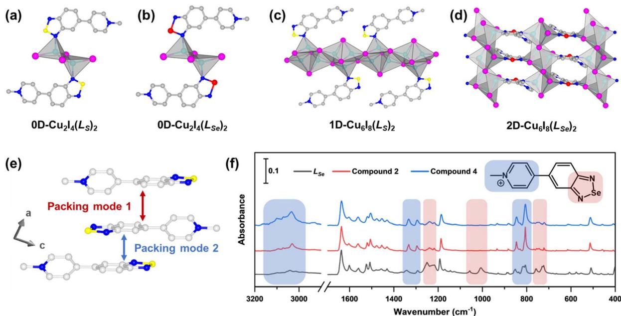
Fig. 1 Crystal structures of compounds (a) 1, (b) 2, (c) 3, and (d) 4. (e) Two different  $\pi$ - $\pi$  packing modes within compound 1, color scheme: cyan: Cu; purple: I; gray: C; blue: N; yellow: S; red: Se. All H atoms are omitted for clarity. (f) Experimental IR spectra of free ligand  $L_{Se}$  (black) and compounds 2 (red) and 4 (blue). The absorbance is normalized to the phenyl-ring stretching band  $\nu(C=C)$  around  $1610\text{ cm}^{-1}$ .
