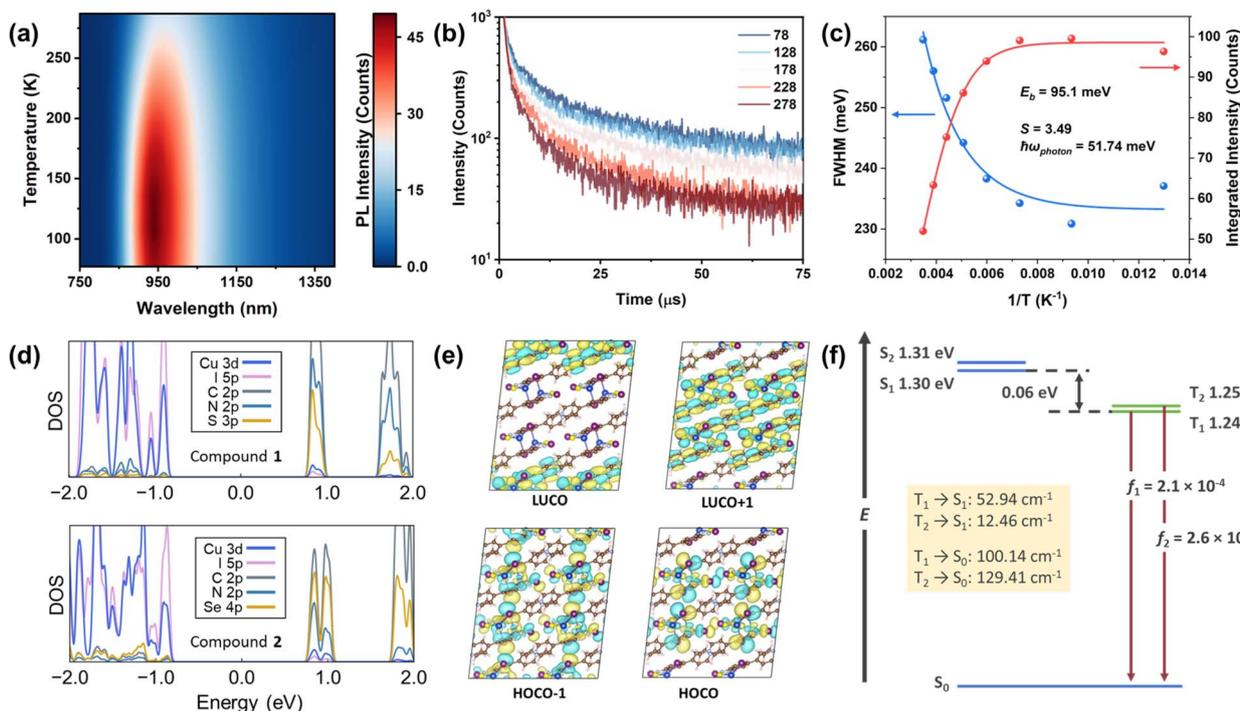
Fig. 3 (a) Temperature-dependent PL spectra, (b) PL decay curves and (c) Huang–Rhys factor ( $S$ ) and exciton binding energy ( $E_b$ ) fittings of compound 1. (d) Calculated projected density of states (PDOS) of compounds 1 and 2. (e) Calculated frontier crystal orbitals and (f) energy level diagram and SOC constant of compound 1.
