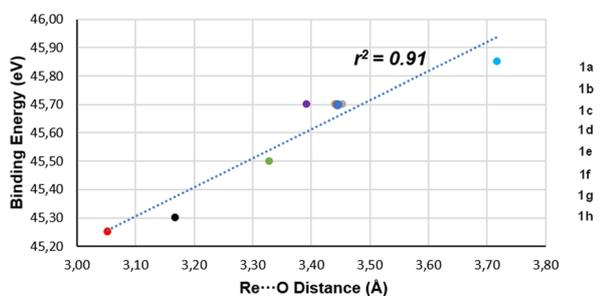
Fig. 4 Correlation between Re 4f<sub>7/2</sub> BE from XPS analysis (the values 45.85, and 45.25 have been used for **1g**, and **1h**) and Re...O distance from single-crystal XRD.
