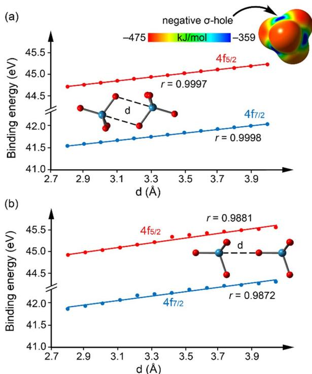
Fig. 6 The molecular electrostatic potential (MEP) surface is shown in the upper part of the figure, with a MEP value of  $-359 \text{ kJ mol}^{-1}$  at the rhenium  $\sigma$ -holes and  $-475 \text{ kJ mol}^{-1}$  at the oxygen atoms. The lower part displays correlation plots (a and b) between the theoretical Re  $4f$  BEs and the corresponding Re...O distances.
