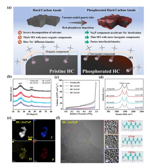
Fig. 1 Synthesis and structural features. (a) Schematic diagram showing the preparation of a phosphorated hard carbon anode and working mechanism of the phosphating layer design. (b) XRD patterns of all as-prepared samples. (c)  $N_2$  adsorption–desorption isotherms. (d) Raman spectra. (e) HAADF-TEM images and element mapping of C, O, and P of HC-3 wt% P. (f) HRTEM images of HC-3 wt% P.
