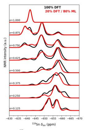
Fig. 8 Simulated <sup>119</sup>Sn NMR spectra of  $La_2(Sn_xZr_{1-x})_2O_7$  obtained using a grand-canonical approach with DFT calculations for all the arrangements in the configurational space (black lines) and predicted with the random forest ML model (red lines), using 20% of the configurations for training.
