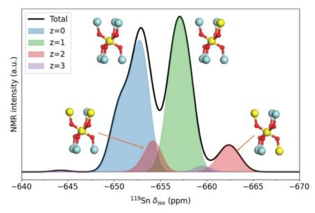
Fig. 6 Decomposition of the  $^{119}$ Sn NMR spectrum of  $La_2(Sn_{0.125}Zr_{0.875})_2O_7$  solid solution (x=0.125), simulated using the grand-canonical ensemble approach, into contributions from given numbers (z) of NNN Sn atoms. In the coordination schemes, Sn atoms are yellow, Zr atoms are blue, and O atoms are small and red.
