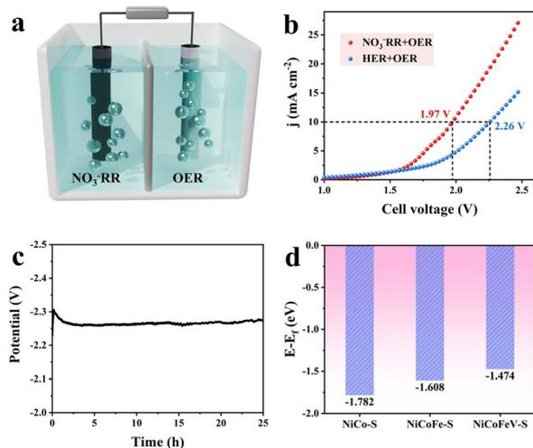
Fig. 5 (a) Two-electrode configuration schematic illustrating simultaneous OER (anode) and nitrate reduction (NO<sub>3</sub>RR, cathode) processes. (b) LSV curves of the electrolyzer under varied conditions: anolyte (1.0 M KOH) and catholyte (1.0 M KOH + 0.1 M KNO<sub>3</sub>). (c) Chronopotentiometric test of the electrolyzer at 10 mA cm<sup>-2</sup>. (d) The statistics of d-band centers for NiCoFeV-S, NiCoFe-S, and NiCo-S.
