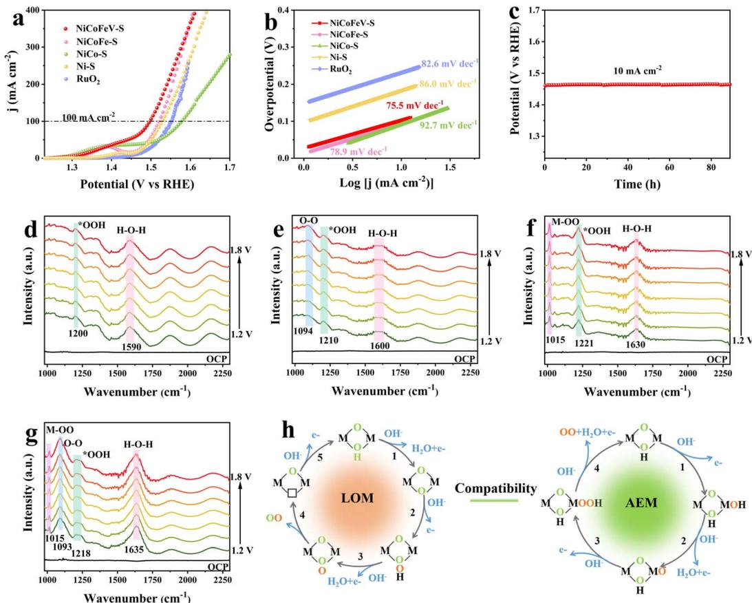
Fig. 2 (a) OER polarization curves and (b) Tafel slopes of samples. (c) Chronopotentiometric response at  $10 \text{ mA cm}^{-2}$  of NiCoFeV-S. *In situ* electrochemical ATR-FTIR spectra of (d) Ni-S, (e) NiCo-S, (f) NiCoFe-S, and (g) NiCoFeV-S under different potential infrared signals. (h) Schematic illustration of the OER pathway over NiCoFeV-S.
