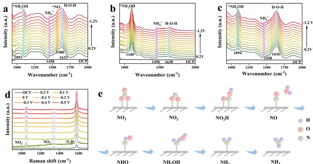
Fig. 4 *In situ* electrochemical ATR-FTIR spectra of (a) NiCo-S, (b) NiCoFe-S, and (c) NiCoFeV-S under different potential infrared signals. (d) *In situ* Raman spectra of NiCoFeV-S at different operation potentials. (e) Schematic illustration of the NO<sub>3</sub>RR pathway.
