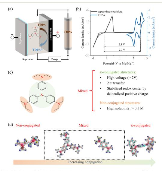
Fig. 1 Scope. (a) Mg RFBs (schematic). (b) CV of the Mg anode reaction and amine-based catholyte reaction. (c) Design principle of amine molecules as the catholyte for Mg RFBs. (d) Electrostatic potential based on the electron density from natural bond orbital analysis<sup>22</sup> in the Gaussian 16 (ref. 23) package. Figures were rendered using Avogadro software.<sup>24</sup> Red indicates higher charge density, and blue indicates lower charge density.
