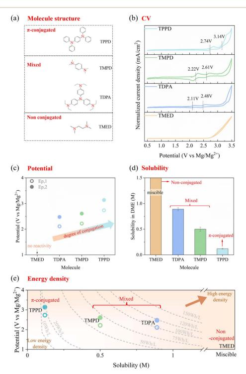
Fig. 3 Structural effect on the electrochemical performances of amine molecules. (a) Molecular structure, (b) CV profile, (c) potential, (d) solubility and (e) theoretical energy density of different amine molecules in the Mg electrolyte. The concentration of active materials was set at 1 mM. Hollow circles and solid circles represent the first pair of peaks and the second pair of peaks, respectively.
