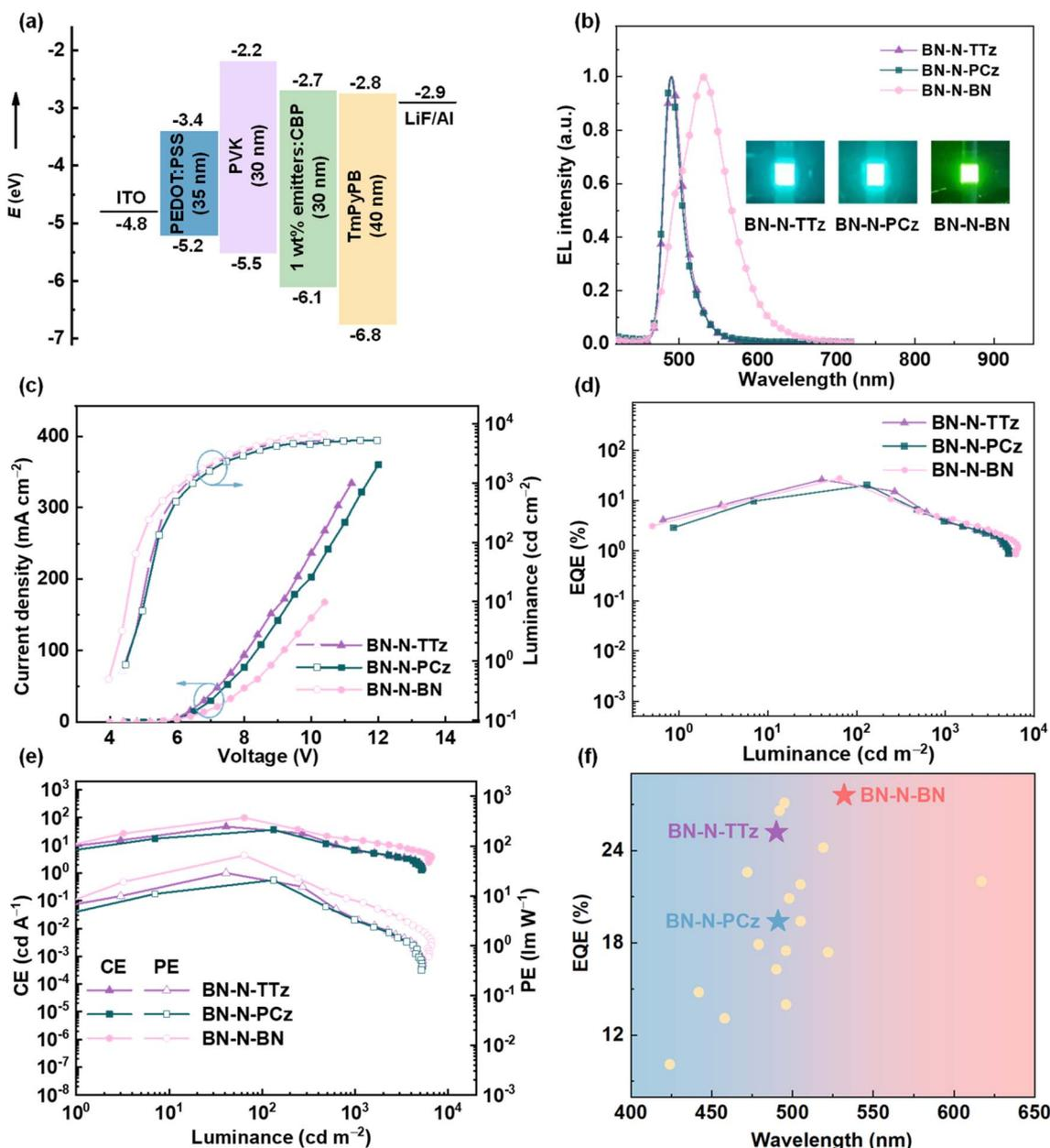
Fig. 7 (a) Device structure. (b) EL spectra of the device (inset: photograph of solution-processed OLEDs based on BN-N-TTz, BN-N-PCz and BN-N-BN). (c) Current density ( $J$ )-voltage ( $V$ )-luminance ( $L$ ) curves. (d) EQE versus luminance characteristics. (e) CE or PE versus luminance characteristics. (f) Maximum EQE of solution-processed OLEDs based on MR-TADF emitters without sensitizers.
