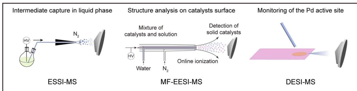
Ambient mass spectrometry (AMS) for online monitoring & mechanistic study
