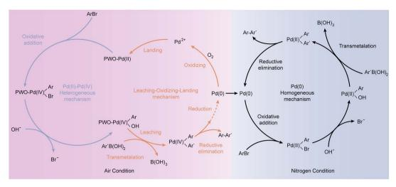
Fig. 5 Catalytic cycles of the Pd(u)-Pd(v) heterogeneous mechanism (blue), the homogeneous mechanism (black), and the leaching-oxidizing-landing mechanism of Pd species (orange).
