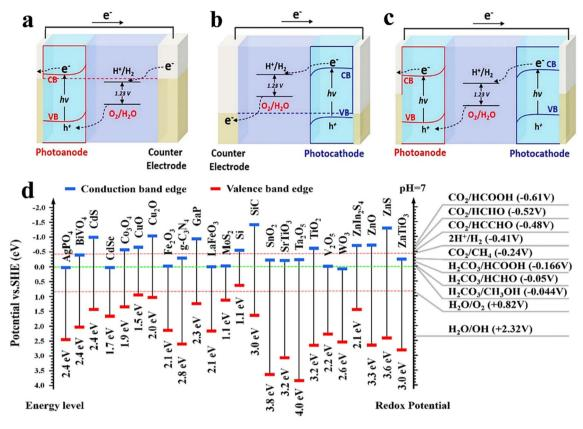
Fig. 2 Schematic illustration of PEC water splitting using (a) a photoanode, (b) photocathode, and (c) a tandem configuration combining both a photoanode and photocathode (reprinted with permission from ref. 30, Copyright 2014 Wiley-VCH Verlag). (d) CB and VB edges of semi-conductor photocatalysts, along with their corresponding redox potentials in aqueous media (reprinted with permission from ref. 33, Copyright 2024 Royal Society of Chemistry).
