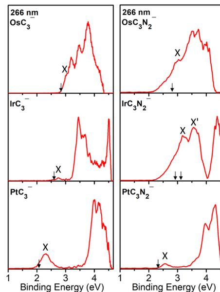
Fig. 1 Photoelectron spectra of  $MC_3^-$  and  $MC_3N_2^-$  ( $M = Os, Ir, Pt$ ) at 266 nm (4.661 eV). Mark X represents the vertical detachment energy, and the black arrow represents the experimentally estimated adiabatic detachment energy.
