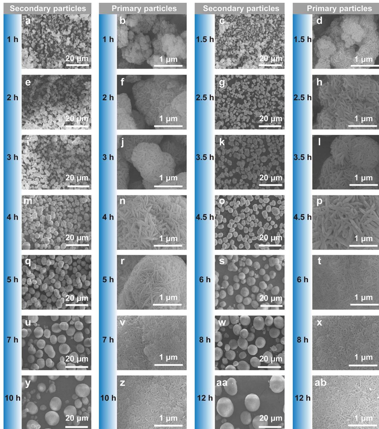
Fig. 2 SEM images of the secondary particles (a–aa) and primary particles (b–ab) for  $\text{Ni}_{0.8}\text{Co}_{0.1}\text{Mn}_{0.1}(\text{OH})_2$  at different reaction times.
