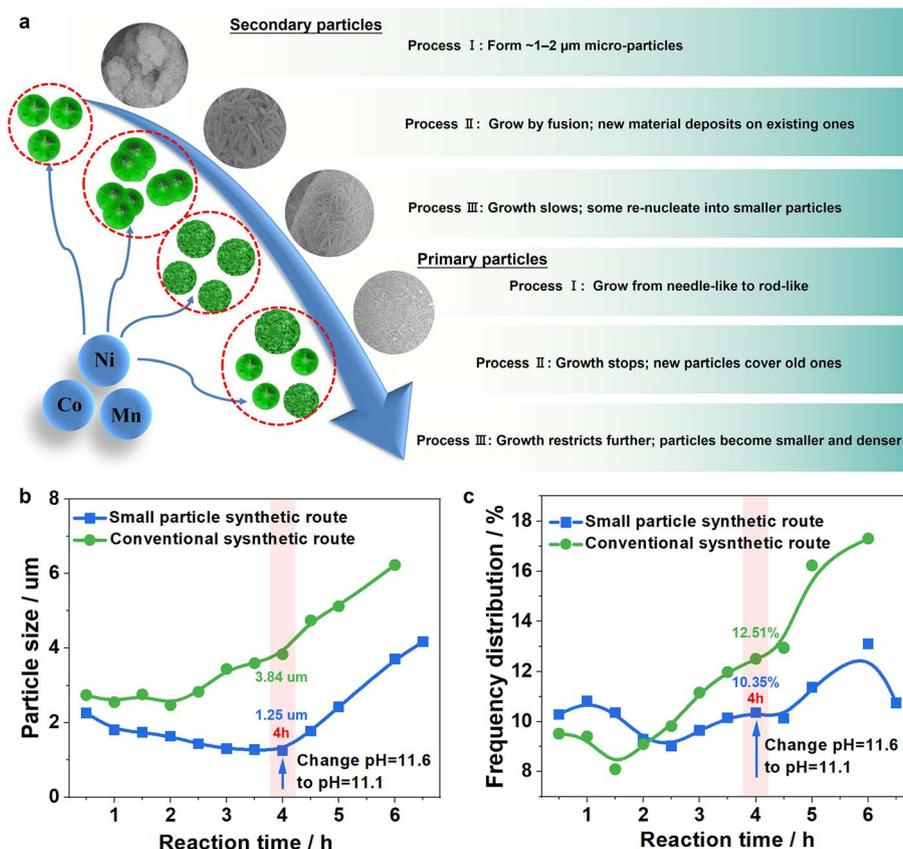
Fig. 4 (a) Growth mechanism of Ni<sub>0.8</sub>Co<sub>0.1</sub>Mn<sub>0.1</sub>(OH)<sub>2</sub>. (b) Overview of particle size evolution at different reaction times. (c) Frequency distribution analysis of Ni<sub>0.8</sub>Co<sub>0.1</sub>Mn<sub>0.1</sub>(OH)<sub>2</sub> at various reaction times.
