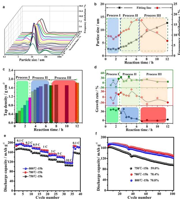
Fig. 3 (a) Particles distribution. (b)  $D_{50}$  and frequency distribution. (c) Tap density. (d) Relative growth rate for  $\text{Ni}_{0.8}\text{Co}_{0.1}\text{Mn}_{0.1}(\text{OH})_2$  at different reaction time. (e) Rate performance for  $\text{LiNi}_{0.8}\text{Co}_{0.1}\text{Mn}_{0.1}\text{O}_2$  at different sintering temperatures. (f) Cycling performance at 1 C for  $\text{LiNi}_{0.8}\text{Co}_{0.1}\text{Mn}_{0.1}\text{O}_2$  at different sintering temperatures.
