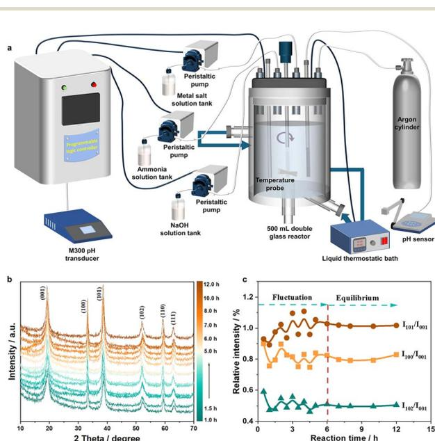
Fig. 1 (a) Schematic diagram illustrating the experimental configuration for precursor synthesis. (b) XRD patterns of  $\text{Ni}_{0.8}\text{Co}_{0.1}\text{Mn}_{0.1}(\text{OH})_2$  at various reaction times. (c) The ratios of XRD characteristic peaks (101)/(001), (100)/(001), (102)/(001) for  $\text{Ni}_{0.8}\text{Co}_{0.1}\text{Mn}_{0.1}(\text{OH})_2$  at different reaction times.
