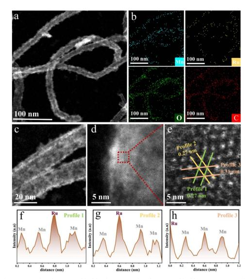
Fig. 1 (a) HAADF-STEM image of CNT-(Mn<sub>0.75</sub>Ru<sub>0.25</sub>)O<sub>2</sub>. (b) EDS mapping of CNT-(Mn<sub>0.75</sub>Ru<sub>0.25</sub>)O<sub>2</sub>. (c) High-magnification STEM image showing the morphology from (a). (d) Atomic-resolution STEM image of a representative part selected from (c). (e) Enlarged view of the red-boxed region in (d). (f-h) The corresponding intensity profile of the line regions in (e).
