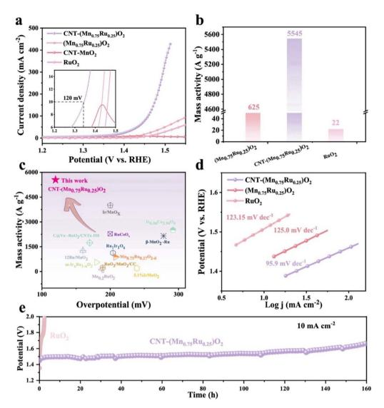
Fig. 3 (a) OER performance of the catalysts in 0.1 M HClO<sub>4</sub> solution. (b) Mass activity at 1.5 V of the catalysts. (c) Comparison of OER overpotential and mass activity of previously reported electrocatalysts. (d) Tafel slope of the catalysts. (e) Durability test of CNT-(Mn<sub>0.75</sub>Ru<sub>0.25</sub>)O<sub>2</sub> and RuO2.
