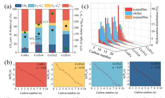
Fig. 2 (a) The catalytic performance of the prepared catalysts. (b) The chain growth factors of the prepared catalysts. (c) The product distribution of the prepared catalysts (reaction conditions: 320 °C, 3 MPa, 9000 mL  $g_{cat}^{-1}$  h<sup>-1</sup>, TOS = 8 h).
