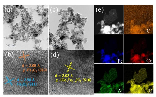
TEM and HRTEM images of the spent (a and b) Co0Fe and (c and d) Co1Fe2 catalysts; (e) elemental mapping of the spent Co1Fe2 catalyst.
