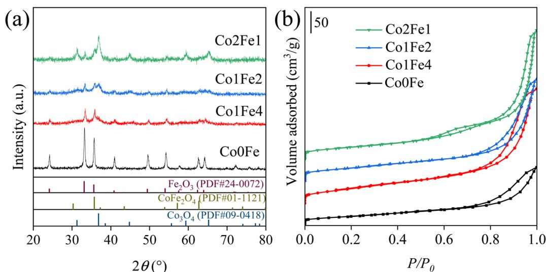
Fig. 1 (a) XRD patterns and (b) N<sub>2</sub> adsorption–desorption isotherms of the prepared catalysts.
