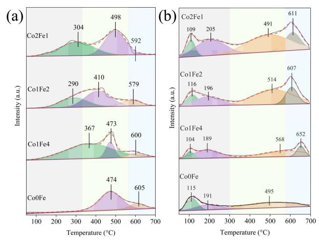
Fig. 7 (a) H<sub>2</sub>-TPD and (b) CO<sub>2</sub>-TPD profiles of the prepared catalysts.
