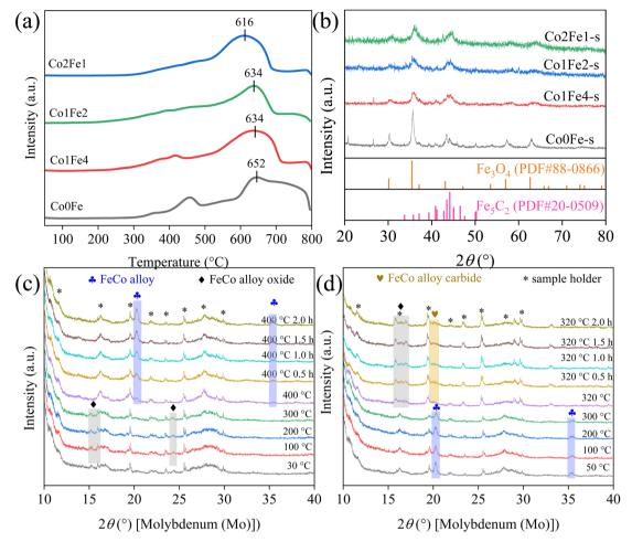
Fig. 4 (a) H<sub>2</sub>-TPR profiles of the prepared catalysts; (b) XRD patterns of the spent catalysts; in situ XRD patterns for the Co1Fe2 catalyst during the (c) reduction and (d) reaction process. "\*" symbol represents the diffraction peaks of sample holder, which is unavoidable because of supporting the samples.
