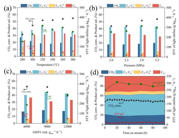
Fig. 3 Effects of (a) reaction temperature, (b) pressure, and (c) GHSV on the catalytic performance of Co1Fe2. (d) The durability test of CO2 hydrogenation over the Co1Fe2 catalyst (reaction conditions: 320 °C, 3 MPa, 9000 mL  $g_{cat}^{-1} h^{-1}$ , TOS = 8 h unless specified).
