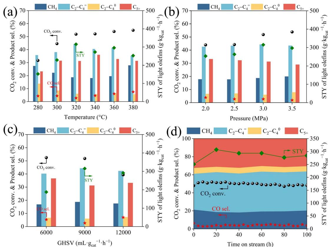
Fig. 3 Effects of (a) reaction temperature, (b) pressure, and (c) GHSV on the catalytic performance of Co1Fe2. (d) The durability test of CO<sub>2</sub> hydrogenation over the Co1Fe2 catalyst (reaction conditions: 320 °C, 3 MPa, 9000 mL g<sub>cat</sub><sup>-1</sup> h<sup>-1</sup>, TOS = 8 h unless specified).
