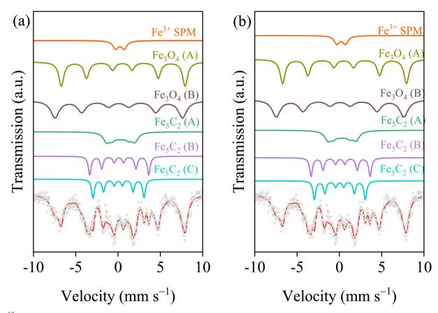
Fig. 6 <sup>57</sup>Fe Mössbauer spectra of the spent (a) Co0Fe and (b) Co1Fe2 catalysts.
