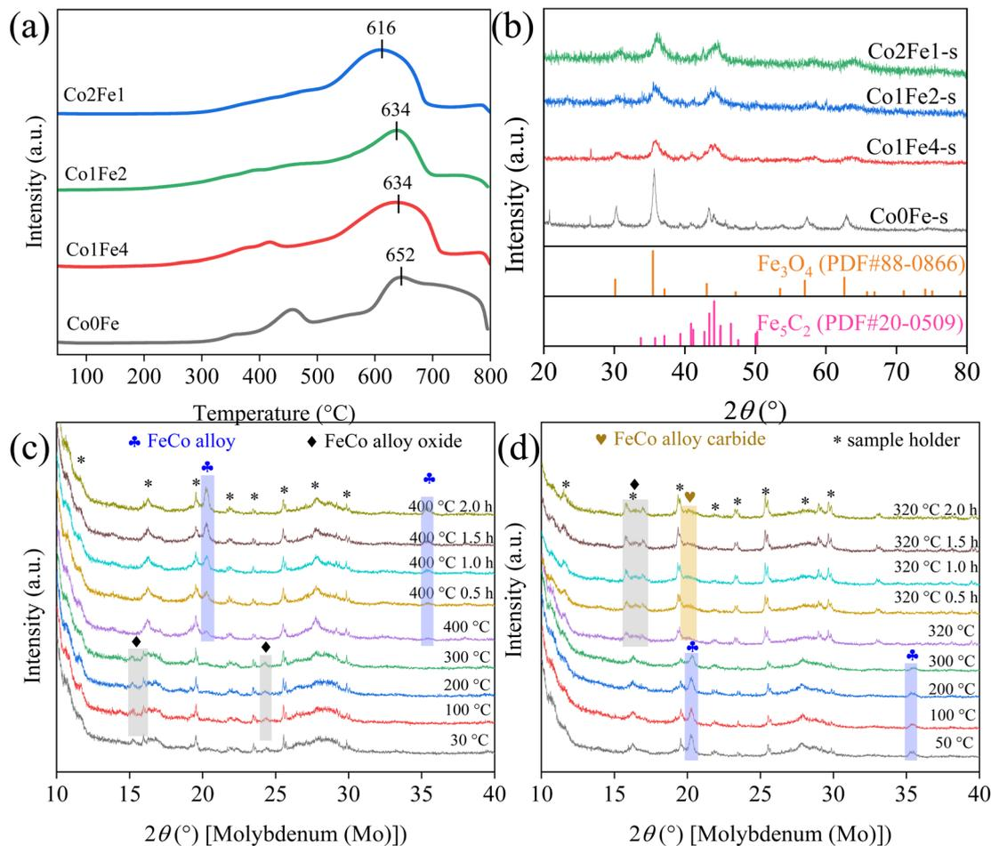
Fig. 4 (a) H<sub>2</sub>-TPR profiles of the prepared catalysts; (b) XRD patterns of the spent catalysts; *in situ* XRD patterns for the Co<sub>1</sub>Fe<sub>2</sub> catalyst during the (c) reduction and (d) reaction process. "\*" symbol represents the diffraction peaks of sample holder, which is unavoidable because of supporting the samples.
