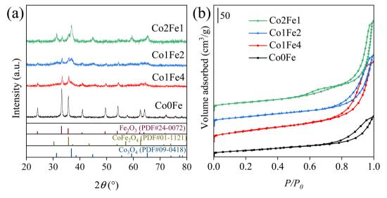
Fig. 1 (a) XRD patterns and (b) N<sub>2</sub> adsorption-desorption isotherms of the prepared catalysts.
