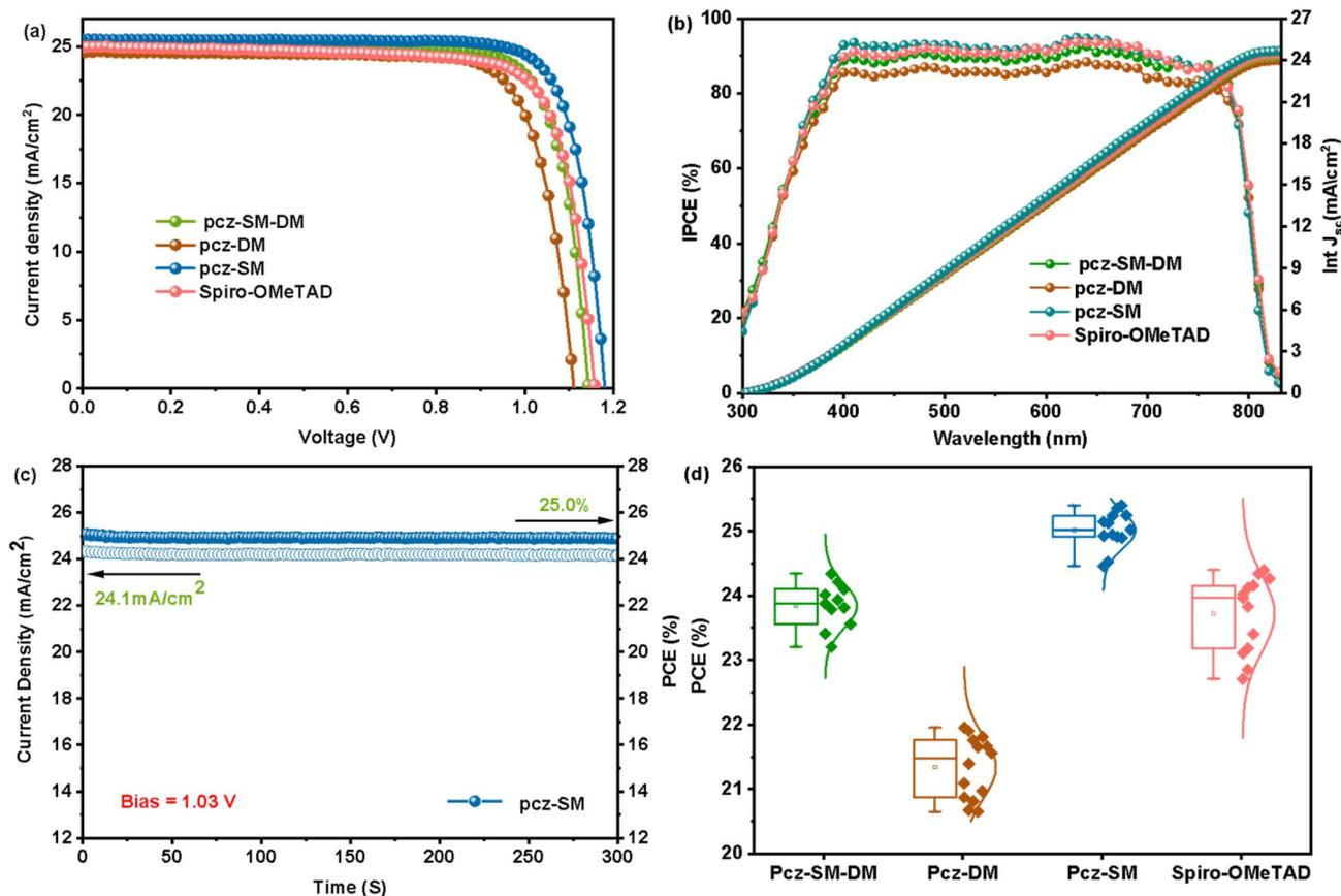
Fig. 3 (a)  $J$ - $V$  curves, (b) IPCE curves and  $J_{sc}$  integration of PSCs containing pcz-SM-DM, pcz-DM, pcz-SM, and Spiro-OMeTAD as HTM. (c) Steady-state PCE of PSCs containing pcz-SM as the HTM at the MPP point, and (d) reproducibility of PSCs based on different HTMs.
