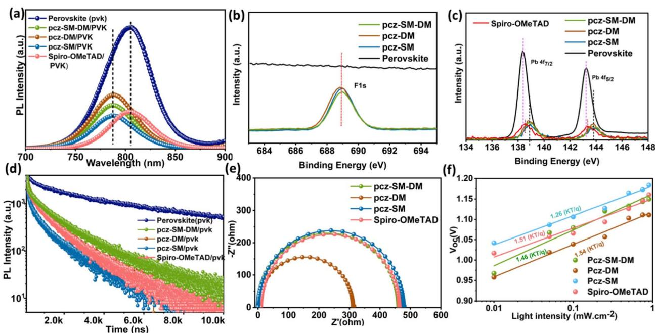
**Fig. 4** (a) Steady-state PL decay curves, (b) F1s XPS spectra and (c) Pb 4f XPS spectra of pristine perovskite, perovskite/pcz-SM-DM, perovskite/pcz-DM, perovskite/pcz-SM, and perovskite/Spiro-OMeTAD, (d) time-resolved PL decay results, (e) Nyquist plot, and (f) light intensity-dependent  $V_{OC}$  behavior of pcz-SM-DM, pcz-DM, and pcz-SM, and Spiro-OMeTAD.
