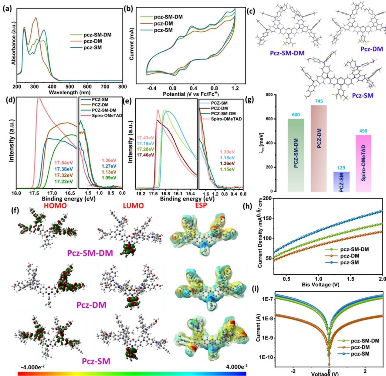
Fig. 1 (a) UV absorption spectra in THF ( $2 \times 10^{-5}$  mol L $^{-1}$ ); (b) CV curve analyses in DCM ( $1.0 \times 10^{-3}$  M); (c) the optimized structures of HTMs; UPS spectra of (d–e) un-doped and doped HTMs in a solid thin film; (f) DFT spatial distribution of HOMO and LUMO levels and ESP; (g) reorganization energy ( $\lambda_{\text{h}}$ ) associated with hole transport, (h) hole mobility, and (i) conductivity of pcz-SM-DM, pcz-DM, and pcz-SM, HTMs.
