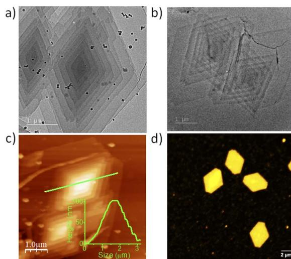
Fig. 1 TEM images of self-assembled **PTZ-P1** exhibiting multi-layered diamond-shaped 2D morphology in (a) iPrOH,  $c = 0.25 \text{ mg mL}^{-1}$ ; (b) 20% iPrOH/water,  $c = 0.05 \text{ mg mL}^{-1}$ ; (c) AFM image (inset: showing the height profile of the nanoplatelets) and (d) CLSM image from a solution of **PTZ-P1** in 20% iPrOH/water mixture;  $c = 0.05 \text{ mg mL}^{-1}$ . (d) CLSM image from a solution of **PTZ-P1** in a 20% iPrOH/water mixture;  $c = 0.05 \text{ mg mL}^{-1}$ .
