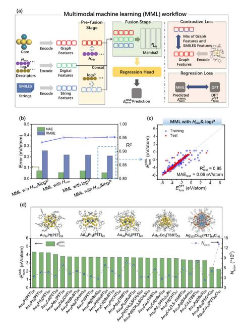
Fig. 4 (a) The flowchart of formation energy prediction on bimetallic nanoclusters by multimodal machine learning; (b) comparison of the performance of the MML models; (c) prediction of formation energy ( $E_{form}$ ) by the MML with log P and  $H_{mix}$ ; (d) prediction of the synthesized bimetallic nanoclusters.
