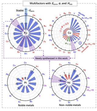
Fig. 8 The accessibility prediction via  $E_{form}$ ,  $\varphi$ , and  $H_{mix}$  for the bimetallic pairs comprising noble metals (Au/M and Pt/M) and base metals (Cu/M and Ni/M) predicted by machine learning.
