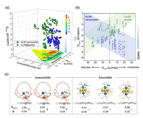
Fig. 6 (a) The formation energy profiles of bimetallic materials with  $\varphi$  and  $H_{\text{mix}}$ ; (b) the pairwise relationship between the formation energy and  $H_{\text{mix}}$ ; (c) the structures of inaccessible Cu/M@zeolites and accessible Au/M nanoclusters.
