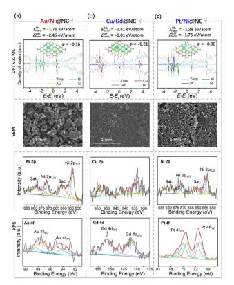
Fig. 10 Plots of DFT vs. ML predicted formation energies and density of states vs. charge density differences; SEM images; and XPS spectra of (a) Au/Ni@NC, (b) Cu/Gd@NC, and (c) Ni/Pt@NC.
