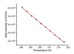
Fig. 5 Variation of the difference in emission intensity at 670 nm for  $[EuL^2]^-$  (5  $\mu$ M) as a function of temperature (50 mM HEPES, 50 mM NaCl, pH 7.4) following successive excitation at 350 and 632 nm; relative thermal sensitivity parameters,  $S_r$  values are 1.6 and 2.6%  $K^{-1}$  at 293 and 318 K respectively. Near identical ( $\pm$ 0.1) values were measured after excitation at 375 and 640 nm.
