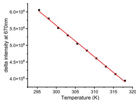
Fig. 5 Variation of the difference in emission intensity at 670 nm for [EuL<sup>2</sup>]<sup>-</sup> (5 μM) as a function of temperature (50 mM HEPES, 50 mM NaCl, pH 7.4) following successive excitation at 350 and 632 nm; relative thermal sensitivity parameters, S<sub>r</sub> values are 1.6 and 2.6% K<sup>-1</sup> at 293 and 318 K respectively. Near identical (±0.1) values were measured after excitation at 375 and 640 nm.
