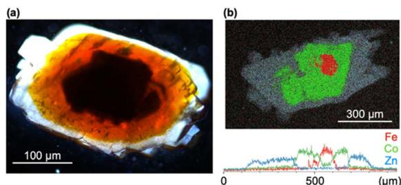
Fig. 5 (a) POM image of  $\text{Fe}_{\text{cdpp}}@_{\text{Co}_{\text{cdpp}}@_{\text{Zn}_{\text{cdpp}}}$ . (b) SEM-EDX elemental map and total area trace along one axis of  $\text{Fe}_{\text{cdpp}}@_{\text{Co}_{\text{cdpp}}@_{\text{Zn}_{\text{cdpp}}}$  after slicing by an ultramicrotome. Color code: iron = red, cobalt = green, zinc = sky blue.
