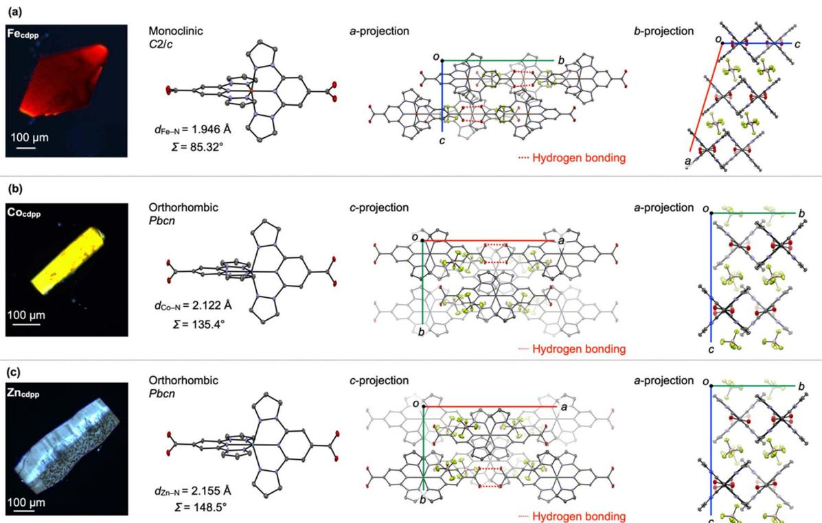
Fig. 2 POM images and X-ray crystal structures (molecular and packing structures) of (a)  $\text{Fe}_{\text{cdpp}}$ , (b)  $\text{Co}_{\text{cdpp}}$  and (c)  $\text{Zn}_{\text{cdpp}}$ . Color code: carbon = gray, nitrogen = blue, oxygen = red, iron = orange, cobalt = purple, zinc = sky blue, fluorine = green, boron = pink. Hydrogen atoms have been omitted for clarity.
