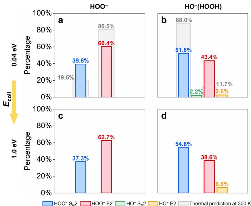
Fig. 2 Branching ratios of the HOO<sup>-</sup>-S<sub>N</sub>2 (blue), HOO<sup>-</sup>-E2 (red), HO<sup>-</sup>-S<sub>N</sub>2 (green) and HO<sup>-</sup>-E2 (orange) pathways for CH<sub>3</sub>CH<sub>2</sub>I reacting with (a and c) HOO<sup>-</sup> and (b and d) HO<sup>-</sup>(HOOH) at collision energies of 0.04 eV (top) and 1.0 eV (bottom).
