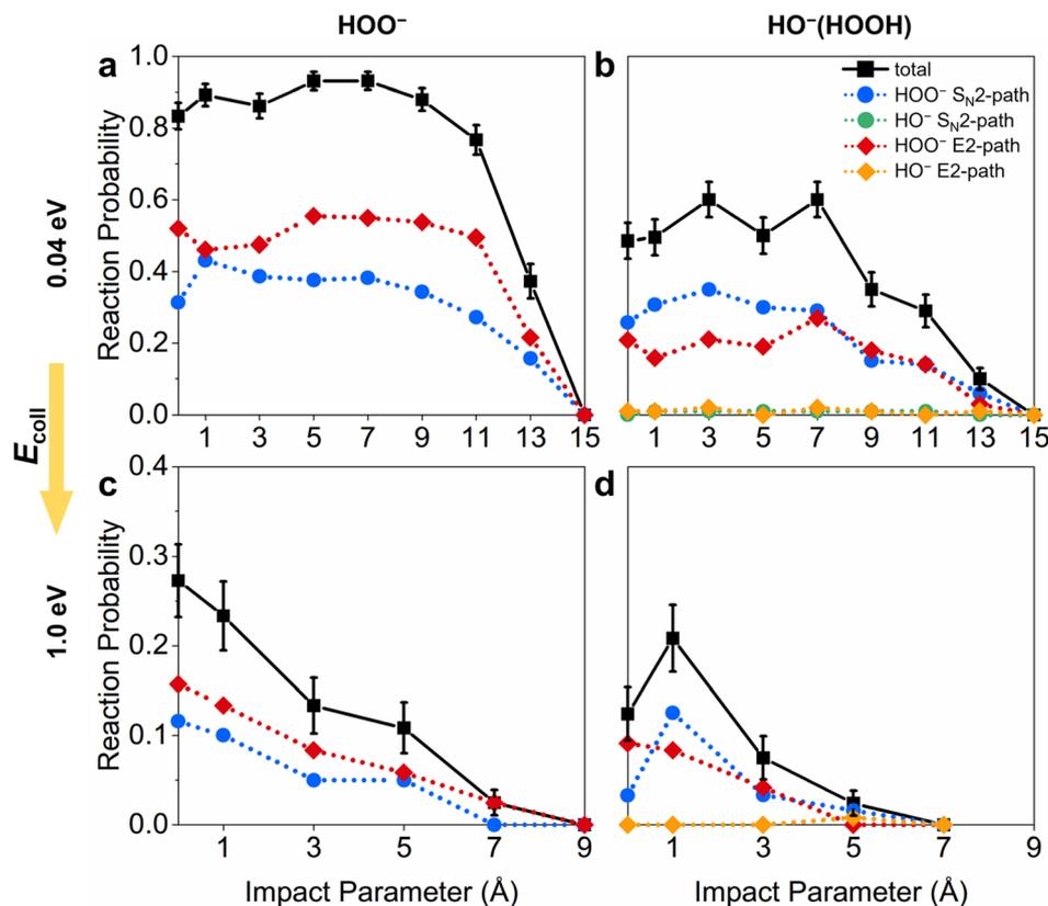
Fig. 1 Opacity functions  $P_r(b)$  of the different pathways for  $\text{CH}_3\text{CH}_2\text{I}$  reacting with (a and c)  $\text{HOO}^-$  and (b and d)  $\text{HO}^-(\text{HOOH})$  at collision energies of 0.04 eV (top) and 1.0 eV (bottom).
