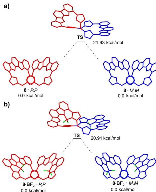
Fig. 5 Theoretical racemization barrier of (a) **8** and (b) **8**·BF<sub>2</sub> calculated at the  $\omega$ B97XD/6-31G(d,p) level of theory.
