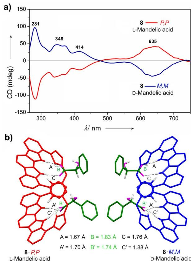
Fig. 6 (a) Chirality induction of **8** upon the addition of *D*- and *L*-Mandelic acid recorded in CH<sub>2</sub>Cl<sub>2</sub> at 298 K, and (b) DFT optimized structures of *P,P* and *M,M* enantiomers of **8** with *L*- and *D*-mandelic acids, respectively.
