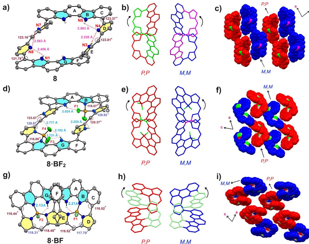
Fig. 2 (a, d and g) X-ray structures of **8**, **8·BF<sub>2</sub>**, and **8·BF**. (b, e and h). *P,P* and *M,M* enantiomers of **8**, **8·BF<sub>2</sub>**, and **8·BF**. (c, f and i) packing of enantiomers in **8**, **8·BF<sub>2</sub>**, and **8·BF**. Meso and *tert*-butyl groups are omitted for clarity (ellipsoid probability level: 60%, grey—C, white—H, orange—boron, blue—N and light green—F).
