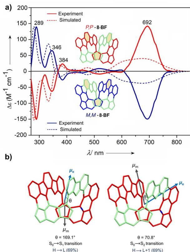
Fig. 4 (a) Experimental and simulated circular dichroism (CD) spectra for (*M,M*)-**8**·BF (blue, first fraction) and (*P,P*)-**8**·BF (red, second fraction) in CH<sub>2</sub>Cl<sub>2</sub>. (b) Angle between the transition dipole moments ( $\mu_e$  and  $\mu_m$ ) at the B3LYP/6-31G(d,p) level of theory.
