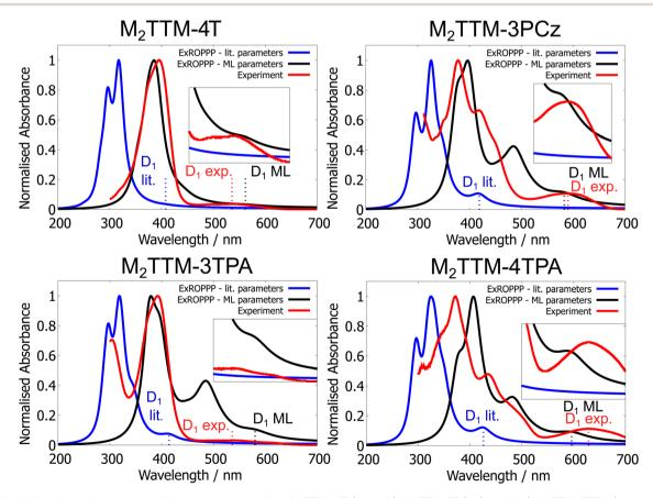
Fig. 8 UV-visible absorption spectra of the newly-synthesised  $M_2TTM-4T$  (top left),  $M_2TTM-3PCz$  (top right),  $M_2TTM-3TPA$  (bottom left) and  $M_2TTM-4TPA$  (bottom right) measured in 0.1 mM toluene solution (red), simulated using ExROPPP with literature parameters (blue) and of the trained 81 molecule ExROPPP model (black). Trained ExROPPP (black) reproduces the experimental spectra (red) more accurately than untrained ExROPPP with literature parameters (blue).
