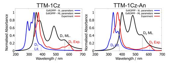
Fig. 5 UV-visible absorption spectra of TTM-1Cz and TTM-1Cz-An measured in 200  $\mu$ M toluene solution at room temperature (red), simulated using ExROPPP with literature parameters (blue) and with the trained 81 molecule model (black). The trained model substantially improves on the literature parameters in both cases.
