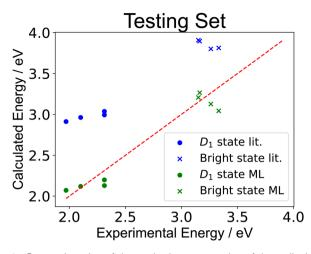
Fig. 9 Regression plot of the excited state energies of the radicals in the testing set calculated by ExROPPP and compared with experimentally determined energies. 'lit.' refers to the parameters sourced from the literature and 'ML' refers to the parameters of the trained 81 molecule model. It can be clearly seen that for this testing set the trained ExROPPP model more accurately reproduces the experimental values than ExROPPP with literature parameters.
