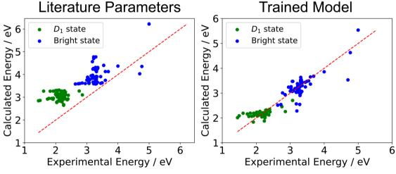
Fig. 4 Regression plots of the excited state energies of the 81 molecule training set calculated by ExROPPP compared with experimentally determined energies, using parameters obtained from the literature (left) and those of the trained ExROPPP model (right). The trained model predicts the energies of UV/visible absorptions much closer to experiment (red line) than do the literature parameters.
