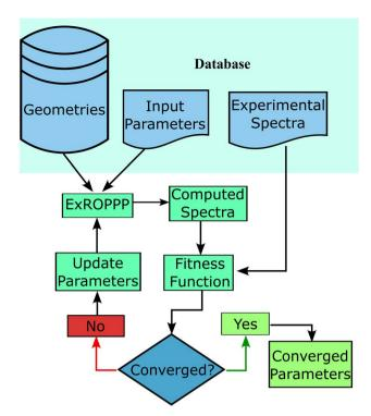
Fig. 3 A flow diagram illustrating our method for training our ExROPPP model on the experimental absorption data of organic radicals.
