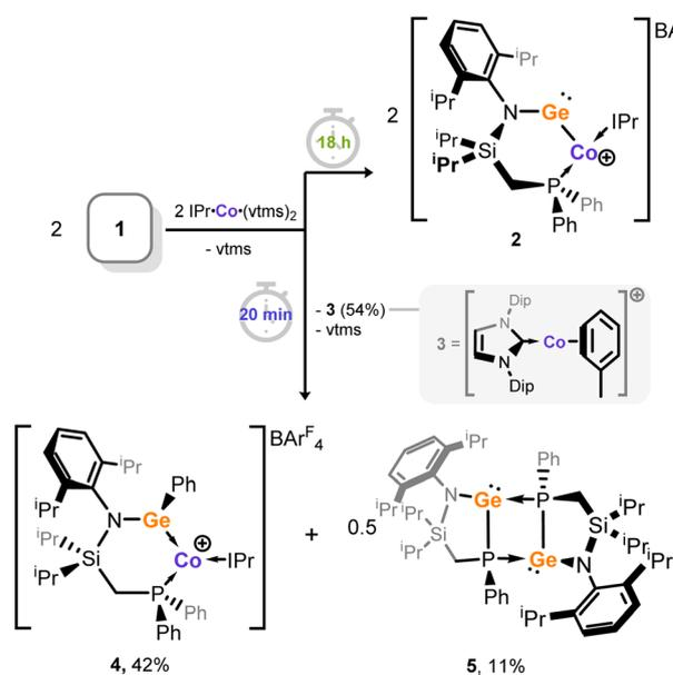
Scheme 2 The formation of species **3**, **4**, and **5** on shortening the reaction time between **1** and  $[\text{IPr}\cdot\text{Co}(\eta_2\text{-vtms})_2]$ , leading to complex fragmentation. Presented yields refer to isolated crystalline solids.
