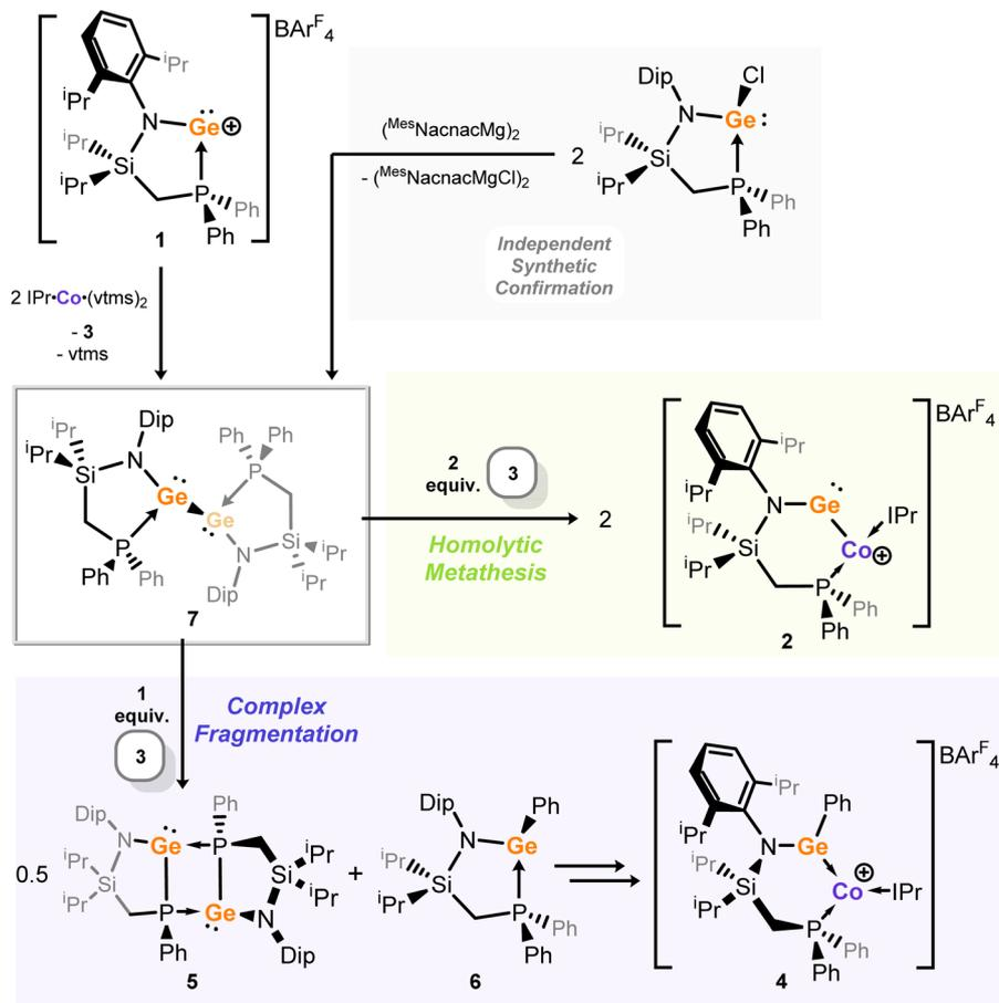
Fig. 6 The reaction map for the initial formation of bis-germylene **7** through reduction of **1** by  $\text{Co}^0$ , (confirmed by its independent synthesis using a dimeric  $\text{Mg}^{\text{I}}$  compound), followed by the stoichiometry-dependent reactivity of **7** towards cationic cobalt species **3**, leading to either cobalto-germylene **2**, or species **4**–**6**.
