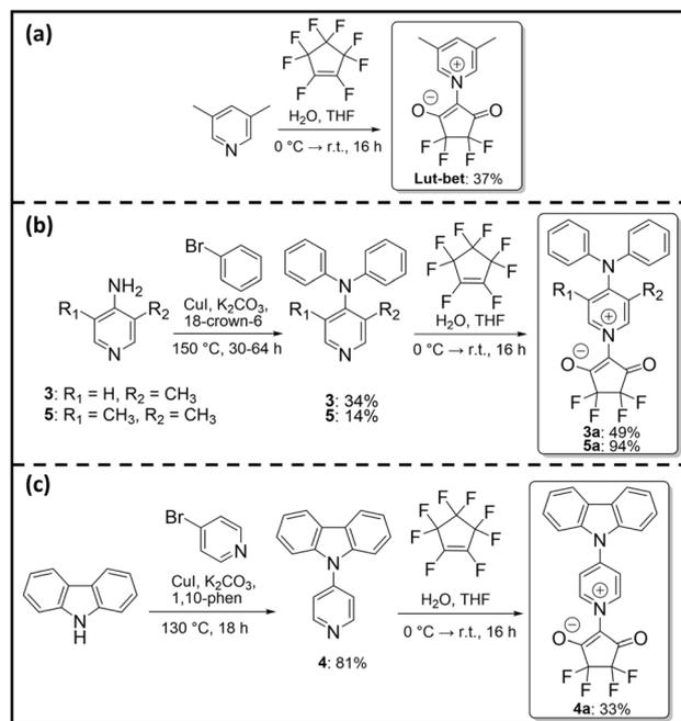
Scheme 1 Synthetic pathway to (a) lutidine betaine (**Lut-bet**); (b) precursors (**3** and **5**) and corresponding betaines (**3a** and **5a**); (c) carbazole precursor (**4**) and corresponding betaine (**4a**).
