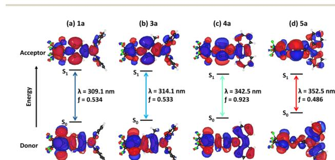
Fig. 7 Natural transition orbitals, vertical transition energies ( $\lambda$ ), and oscillator strengths ( $f$ ) calculated in the gas phase for the  $S_0 \rightarrow S_1$  transition in (a) **1a**; (b) **3a**; (c) **4a**; and (d) **5a**. Calculations were performed at the  $\omega\text{B97xD3}$  def2-TZVP level, on crystal coordinates. Iso-surface values are 0.01.
