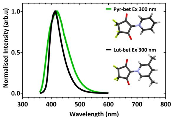
Fig. 2 Solid-state crystalline fluorescence spectra of dried Pyr-bet ( $\lambda_{\text{max}}$  420 nm) and Lut-bet ( $\lambda_{\text{max}}$  414 nm). Inset: excitation wavelengths and depictions of their structures determined by SC-XRD. Spectra are cut above double the excitation wavelength.
