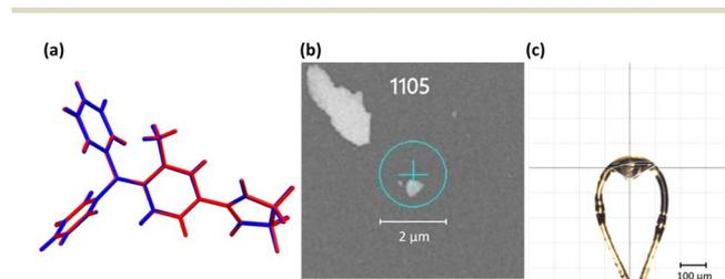
Fig. 6 (a) Electron diffraction and SC-XRD structure overlay for **3a** – ED (red) and SC-XRD (blue); (b) visual image of representative grain used for ED data collection; (c) visual image of crystal used for SC-XRD. Note the scale bars.
