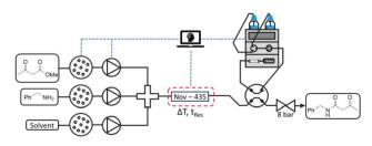
Fig. 1 Self-optimising flow reactor controlled via MATLAB code.
