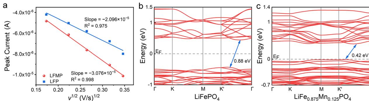
Fig. 2 (a) Plots of the current of the reduction peak ( $I_p$ ) of LFMP and LFP versus the square root of the electrode scanning rate ( $v^{1/2}$ ). Energy band diagrams of LFP (b) and  $\text{LiFe}_{0.875}\text{Mn}_{0.125}\text{PO}_4$  (c).
