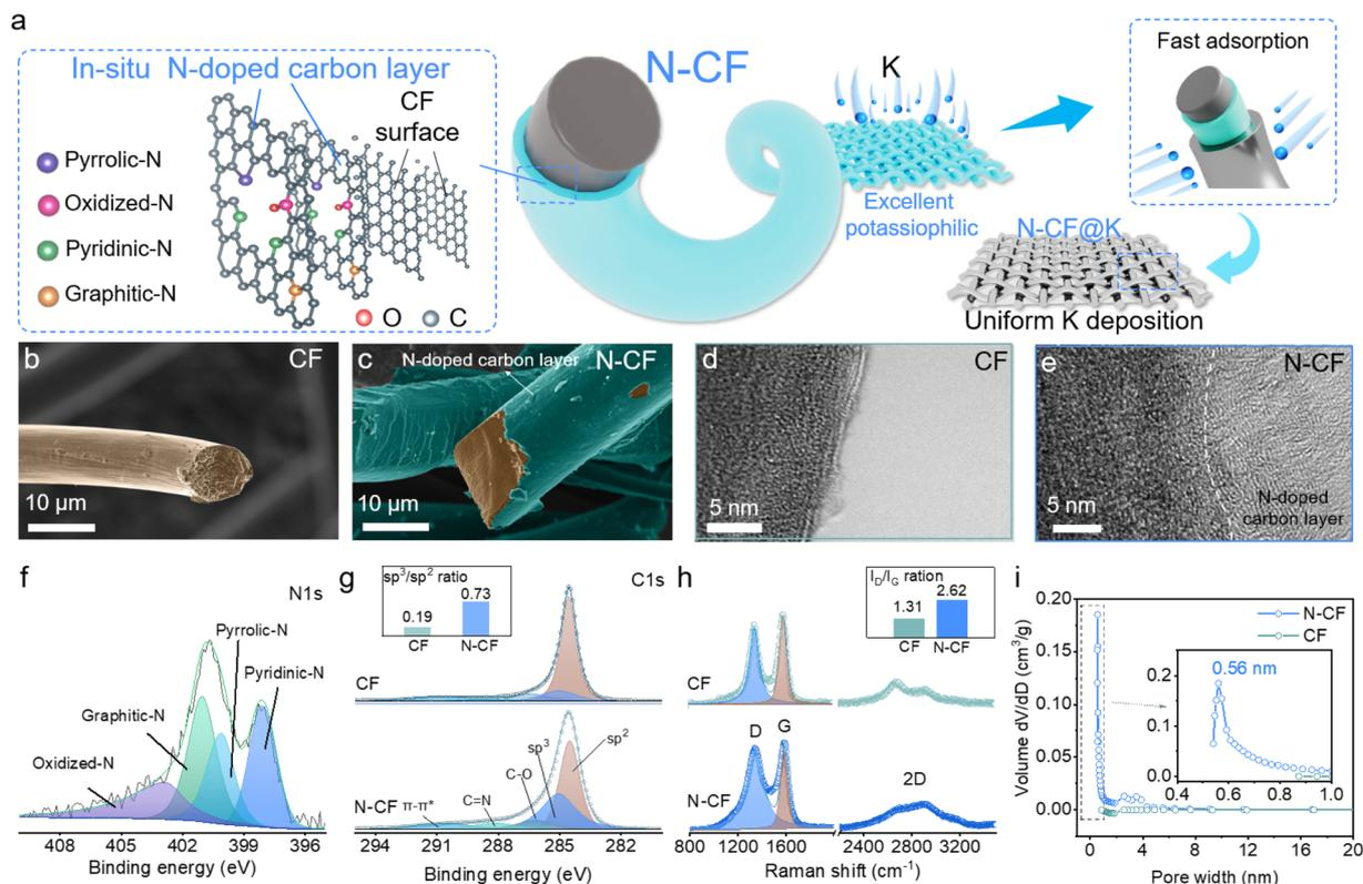
Fig. 1 Schematic and characterization of the potassiophilic N-CF mechanism. (a) Schematic of the K deposition on the N-CF host; (b) SEM images of CF and (c) N-CF; TEM images of (d) CF and (e) N-CF interfaces; (f) XPS N 1s spectrum of N-CF; (g) XPS C 1s spectra of CF and N-CF; (h) Raman spectra and (i) BJH pore size distribution of CF and N-CF.
