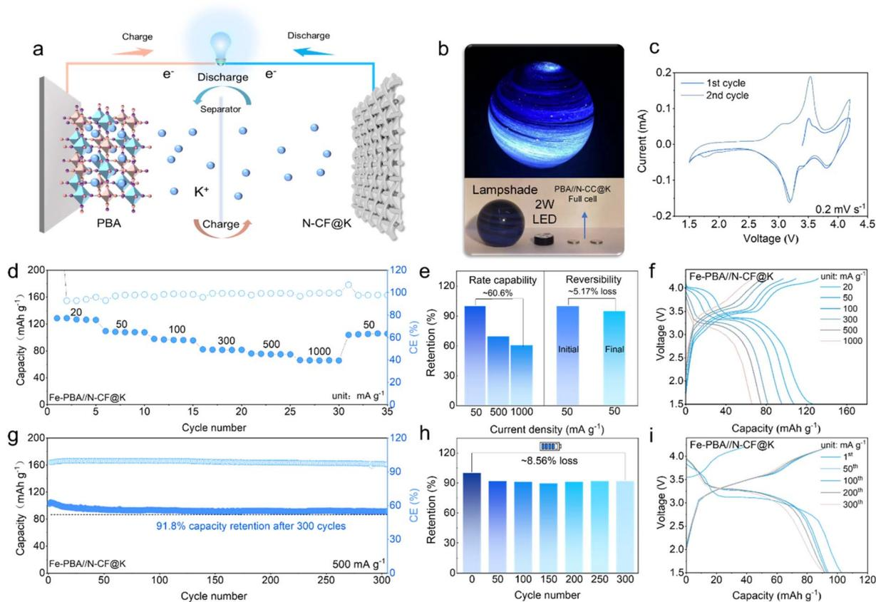
Fig. 5 Electrochemical performance of the PBA||N-CF@K full cell. (a) Schematic diagram; (b) application demonstration; (c) CV curve; (d) rate performance and (e) rate capacity retention statistics; (f) corresponding GCD curve; (g) long-term cycle performance; (h) capacity retention statistics; (i) corresponding GCD curves.
