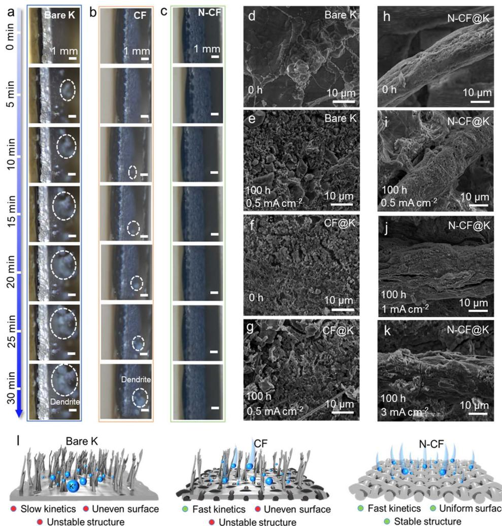
Fig. 4 Process and mechanism of the K metal plating–stripping process. *In situ* optical microscope photographs for (a) bare K, (b) CF@K and (c) N-CF@K at a plating areal current density of  $0.6 \text{ mA cm}^{-2}$ . SEM images of (d and e) bare K, (f and g) CF@K and (h–k) N-CF@K before and after cycling; (l) schematic diagram of the deposition kinetics for bare K, CF, and N-CF.
