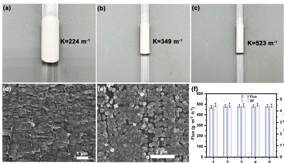
Fig. 5 (a–c) Photographs of the UiO-66/PP-(96) membrane after bending with glass rods of varying diameters,  $K$  is the curvature of bending; (d) cross-section SEM image of the UiO-66/PP-(96) membrane; (e) top-view SEM image of the UiO-66/PP-(96) membrane; (f) total flux and *n*-Hex/22DMB separation factor of the UiO-66/PP-(96) membrane after bending 5 times.
