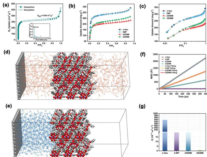
Fig. 1 (a)  $N_2$  adsorption–desorption isotherm measured at 77 K for UiO-66 and the pore size distribution; adsorption isotherms of hexane isomers: (b) linear and (c) logarithmic scale of *n*-Hex, 2MP, 23DMB and 22DMB for UiO-66. The diffusion behaviors of (d) *n*-Hex (orange) and (e) 22DMB (blue) on UiO-66 obtained by MD simulation; (f) MSD plots of *n*-Hex, 2MP, 23DMB and 22DMB in UiO-66; (g) self-diffusion coefficient of *n*-Hex, 2MP, 23DMB and 22DMB in the UiO-66 material.
