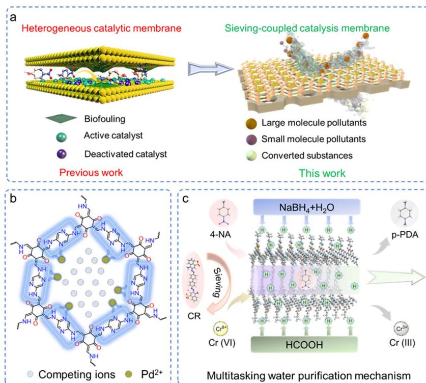
Fig. 1 (a) Comparison of separation synergistic catalytic membranes and heterogeneous catalytic membranes, (b) schematic diagram of capturing  $\text{Pd}^{2+}$  using TpPz membranes, and (c) schematic diagram of the  $\text{Pd}^0$ -TpPz separation synergistic catalytic mechanism.
