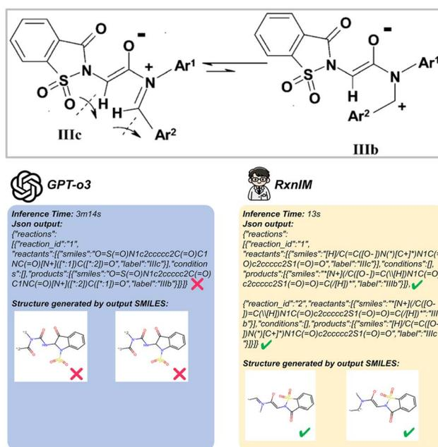
**Fig. 5** Visualization examples of the final JSON output compared to GPT-o3. This example compares RxnIM and GPT-o3 on a reversible reaction image. RxnIM completes inference in 13 s, correctly outputs both reaction directions in JSON with accurate SMILES including aromaticity and formal charges. In contrast, GPT-o3 requires over 3 min, returns only one reaction direction with incorrect SMILES, and fails to capture the correct chemical structure.
