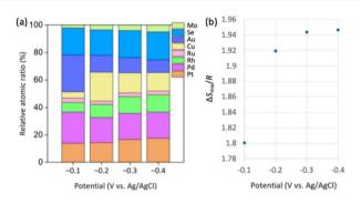
Fig. 5 (a) Relative molar compositions of elements (determined by ICP analysis, as shown in Table S3) and (b) corresponding mixed configuration entropy values ( $\Delta S_{mix}$ ) at different deposition potentials.
