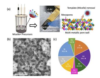
Fig. 1 (a) Fabrication of m-HEA thin films using polymeric micelle templates and their structural illustration. (b) Top-view SEM image and (c) elemental molar composition chart of the m-HEA film.
